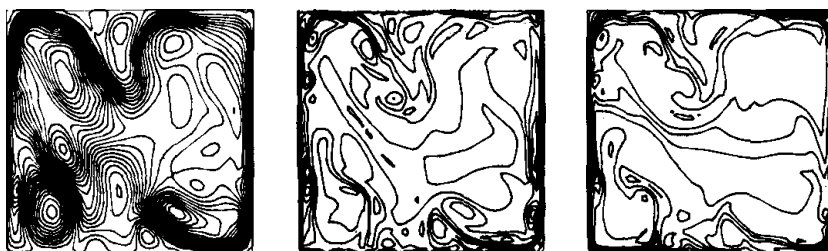
From left to right: instantaneous streamlines, vorticity and isotherms for the buoyant flow in a square box at a Ra number of 10^8 .
