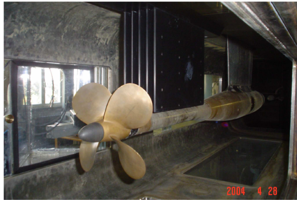
E779A, tunnel set-up. Picture taken from [1].
