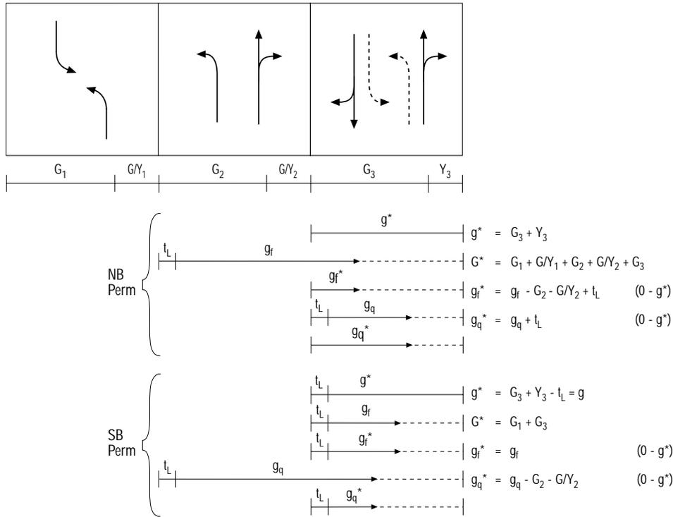
The effective green time for the permitted phase,  $g^*$ , is equal to  $G_2 + Y_2$  for the NB direction and  $G_2 + Y_2 - t_L$  for the SB direction. Note that there is no lost time for the NB movements, since both were initiated in the leading phase, and the lost time is assessed there. Thus, the NB and SB effective green times that must be used are not equal.
