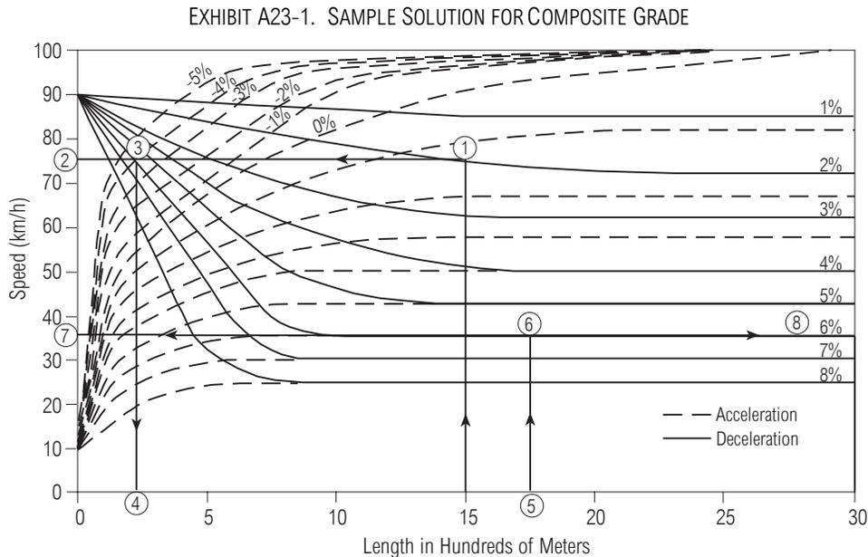
The intersection of the horizontal line with the 6 percent deceleration curve is Point 3. A vertical line is drawn at this point to intersect with the horizontal axis, Point 4. Point 4 indicates that 75 km/h is the speed as if the truck has traveled 225 m on a 6 percent upgrade from level terrain.
