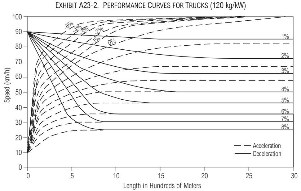
The composite grade procedure is not applicable in all cases, especially if the first segment is downgrade and the segment length is long, or the segments are too short. In using the performance curves, cases that cannot be solved with this procedure will become apparent to the analyst because lines will not intersect or points will fall outside the limits of the curves. In such cases, field measurement of speeds should be used as input to the selection of appropriate truck equivalency values.
