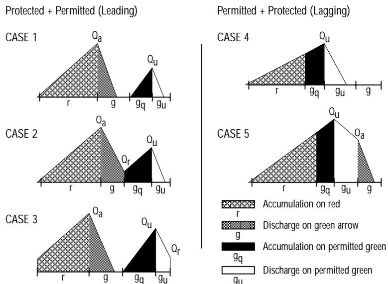
It is first necessary to distinguish between protected-plus-permitted (leading left-turn) phasing and permitted-plus-protected (lagging left-turn) phasing. Three of the five cases shown in Exhibit E16-1 are associated with leading left-turn phases and the other two with lagging left-turn phases. The five cases are identified as follows:
