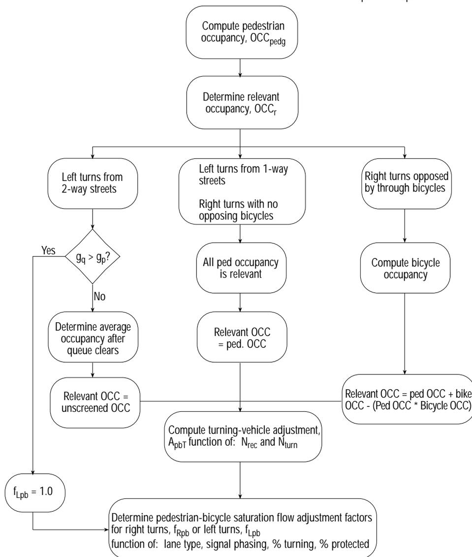
• If the number of cross-street receiving lanes exceeds the number of turning lanes, turning vehicles will more likely maneuver around pedestrians or bicycles and pedestrian-bicycle effects on saturation flow are reduced. The adjustment factor can be calculated using Equation D16-10.
