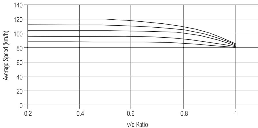
For a rural freeway, the capacity per lane is 2,400 pc/h/ln, based on the assumption that rural freeways have interchange spacing of greater than 3.0 km and two lanes in one direction. Exhibit 23-15 can be used to determine capacity for urban freeways with shorter interchange spacing or a different number of lanes.
