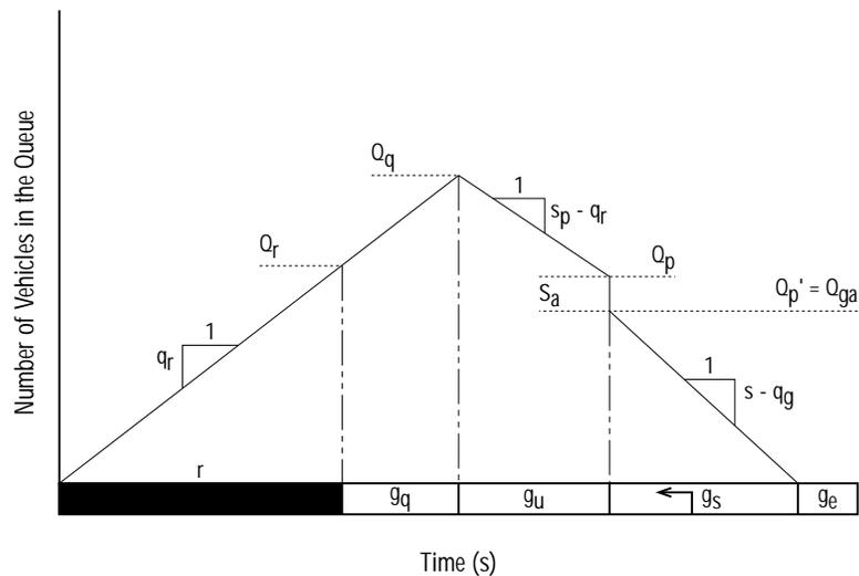
The shape of each QAP is based on termination by a gap that exceeds the unit extension, allowing the full extension time,  $g_e$ , to be displayed. When a phase terminates on the maximum green time, the extension time may be reduced or eliminated. If a permitted left-turn phase terminates before the queue has been served, a maximum of two sneakers will be discharged from the queue at that point.
