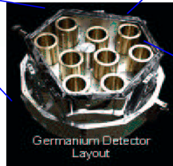
9 segmented coaxial Ge detectors, 7cm x 8.5cm
