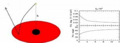
Figure 11. The degree and angle of polarization of the reflected radiation (right panel) as a function of the height of the primary source, assumed for simplicity to be a point on the Black Hole axis (left panel). Such a simple geometry seems able to explain the otherwise puzzling variability of the relativistic iron line in MCG-6-30-15 (Miniutti et al. 2003).
