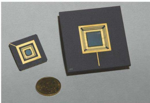
Figure 4. VLSI read-out chips of generation I(2100)pixels and II (20000 pixels)
