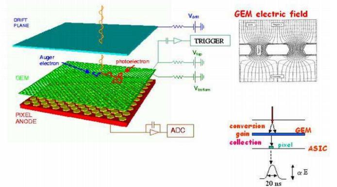
Figure 1. The Concept of Micropattern Gas Chamber
