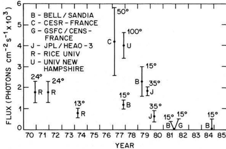
**Fig. 9** The time behaviour of the 511 keV positron annihilation line from the Galactic Center region since its first discovery to 1984 November 20. The FOV of the instruments used is also reported, because there was the suspect that the line intensity could be correlated with the instrument FOV and thus that it could come from an additional source or that the source could be spatially extended (Dunphy et al. 1983). Reprinted from Leventhal et al. (1986).
