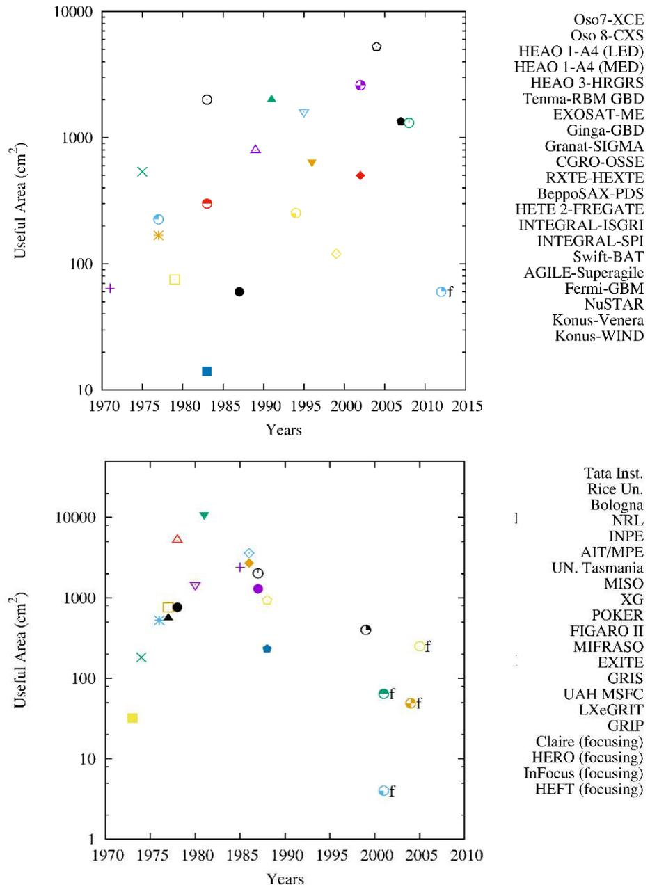
**Fig. 20** Trend with time of the useful area, defined as the geometrical area through the collimator or coded mask, of the hard X-ray non-focusing instruments. In the case of focusing instruments (marked with "f"), it is shown the trend with time of the effective area. *Top panel:* Satellite instruments. Data are taken from Table 1. *Bottom panel:* balloon instruments. Data are taken from Table 2.
