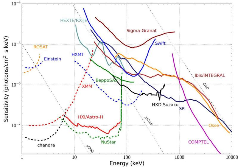
**Fig. 21** Three sigma sensitivity, for an exposure time  $T = 10^5$  s and a bandwidth  $\Delta E = E/2$ , of the most relevant missions in the hard X-ray/soft gamma-ray band. Adapted from Virgili et al. (2017).
