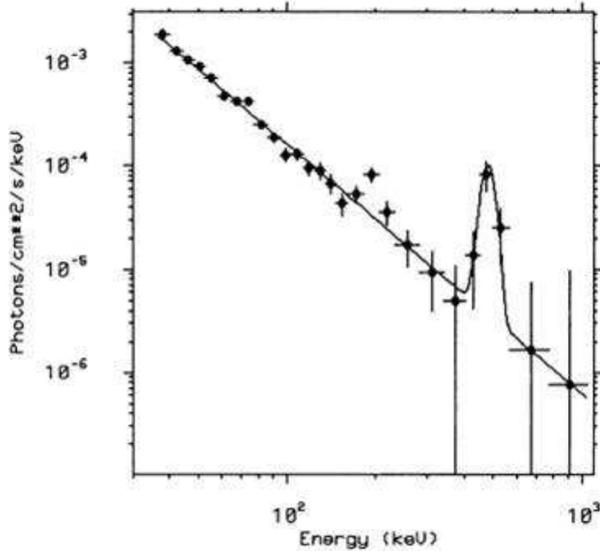
**Fig. 12** First observation of a 480 keV emission line from a point-like source (Nova Muscae) with the SIGMA telescope, interpreted by the observers as a likely redshifted positron annihilation line. Reprinted from Goldwurm et al. (1992).
