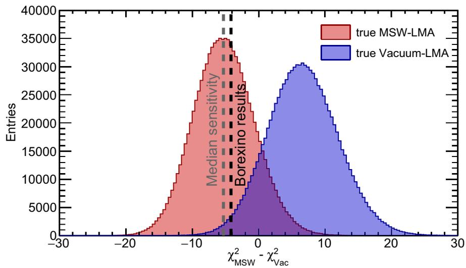
**Extended Data Fig. 2 | Frequentist hypothesis test of MSW-LMA versus vacuum-LMA.** The probability distribution of the test statistics  $t$  is obtained by simulating thousands of sets of  $P_{ee}$  values (at the  $pp$ ,  ${}^7\text{Be}$ ,  $pep$
