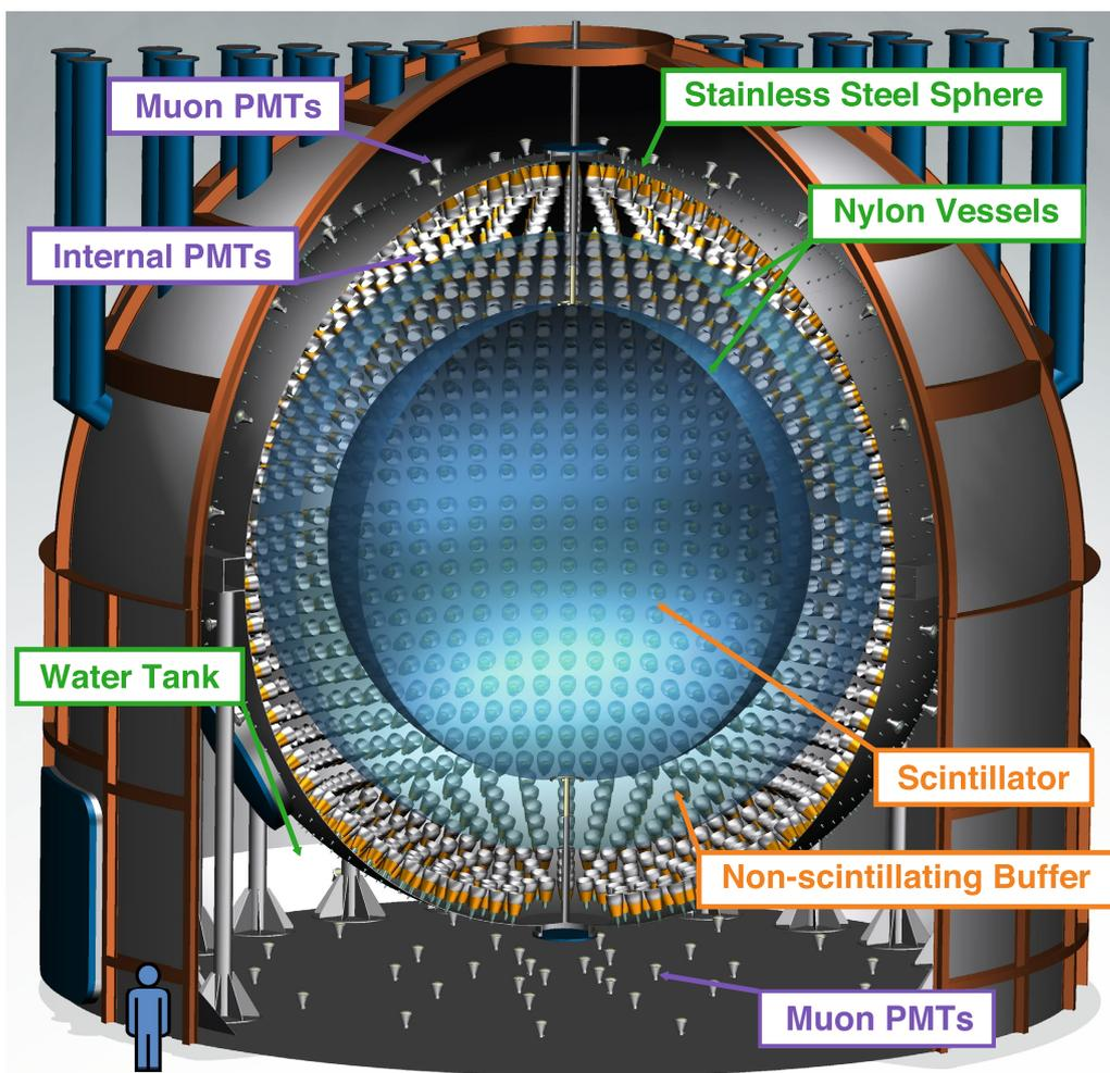
**Extended Data Fig. 1 | The Borexino detector.** Schematic view of the 'onion-like' structure of the Borexino apparatus. From outside to inside: the external water tank; the Stainless Steel Sphere, where about 2,200
