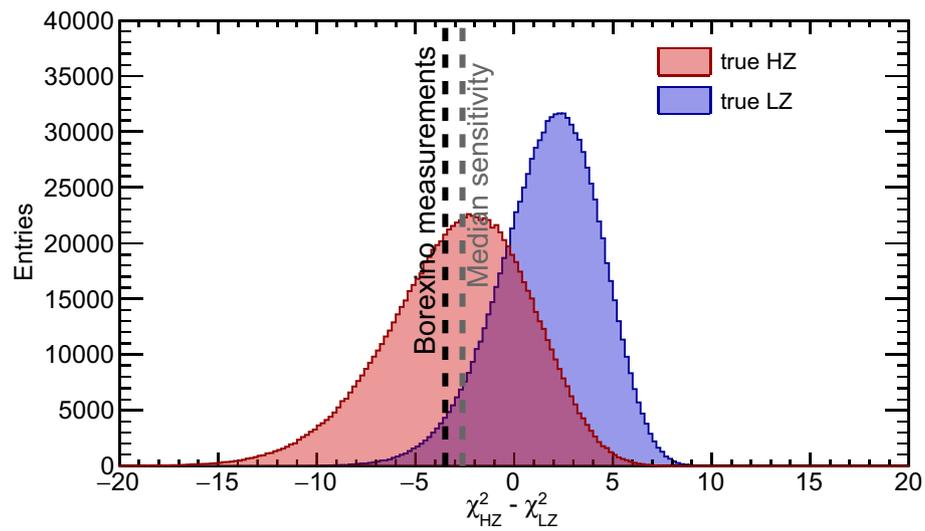
**Extended Data Fig. 3 | Frequentist hypothesis test for LZ and HZ.** The probability distribution of the test statistics  $t$  is obtained by simulating thousands of fake sets of  ${}^8\text{B}$ - ${}^7\text{Be}$  values in the HZ hypothesis (red curve
