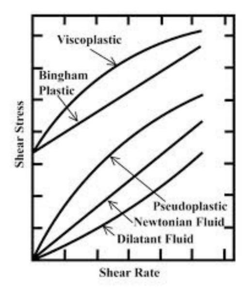
**Shear thinning** is an effect where a fluid's viscosity-the measure of a fluid's resistance to flow decreases with an increasing rate of shear stress. Another name for a shear thinning fluid is a pseudoplastic. This property is found in certain complex solutions, such as lava, ketchup, whipped cream, blood, paint, and nail polish
