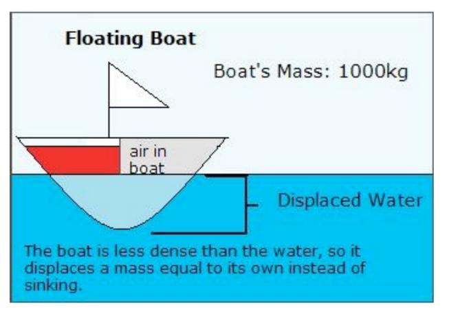
A block of iron dipped in water will sink, while the same metal block shaped like a boat will float.
