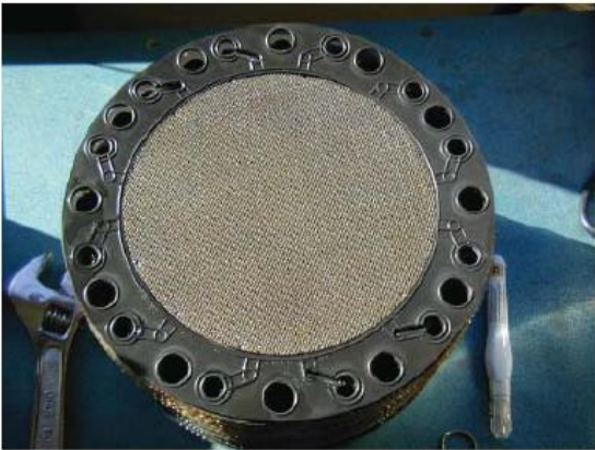
Figure 3.15 Photograph of a grid spacer installed in a rack + details of water injection/gas collection.
