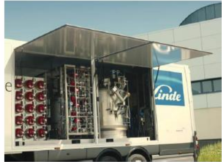
Figure 7.4 Linde mobile refuelling unit. (By kind permission of Linde AG, Germany.)
