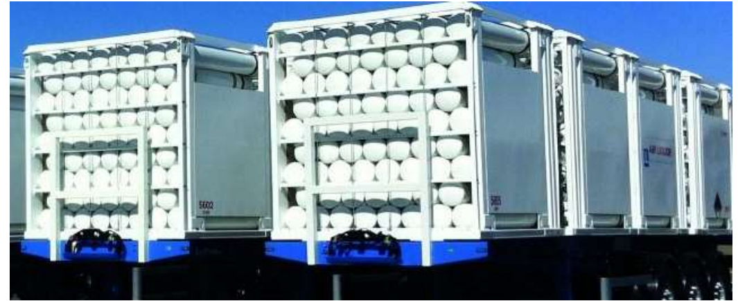
Multiple Element Gas Container (Calvera company)
