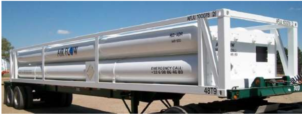
Example of a tube trailer in a 40-foot container half height [49]
