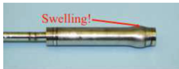
Fig. 6 – Swelling of a 316L stainless steel reactor vessel produced by pressure–temperature cycling of 15 g of LaNi_{4.78}Sn_{0.22}H_x [R.C.Bowman, Jr, previously unpublished].
