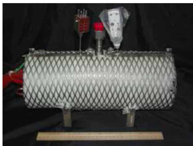
Fig. 18 – A 3-stage metal hydride (LaNi 4.5 Al 0.5 , LaNi 4.9 Al 0.1 , and TiCr 1.8 ) compressor fabricated at the tritium facility of the Savannah River Site (Aiken SC USA) for compression of hydrogen isotopes to pressures of ~620 bar.
