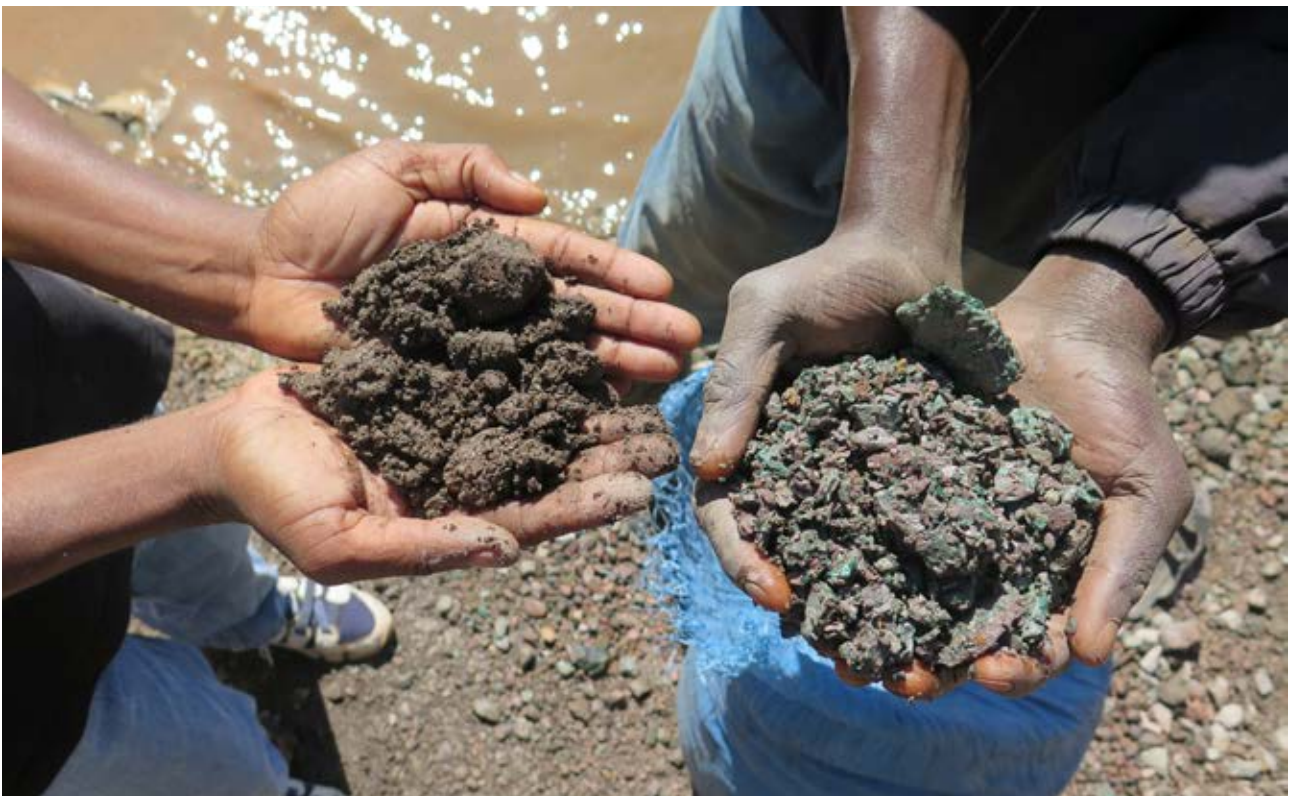
Artisanal miners hold up handfuls of cobalt ore (left) and copper ore (right) that they have scavenged from the mounds of tailings from active and inactive industrial mine sites near Lake Malo, Kapata on the outskirts of Kolwezi, in the DRC. The miners must then sort, wash and crush the mineral ore before selling it to buying houses, May 2015. © Amnesty International and Afrewatch
