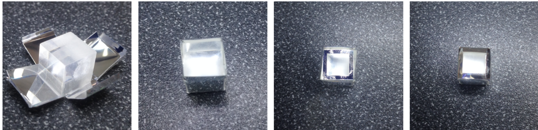
Figure 7: From left to right, the CsI(Tl) crystal wrapping process with Vikuiti ESR.
