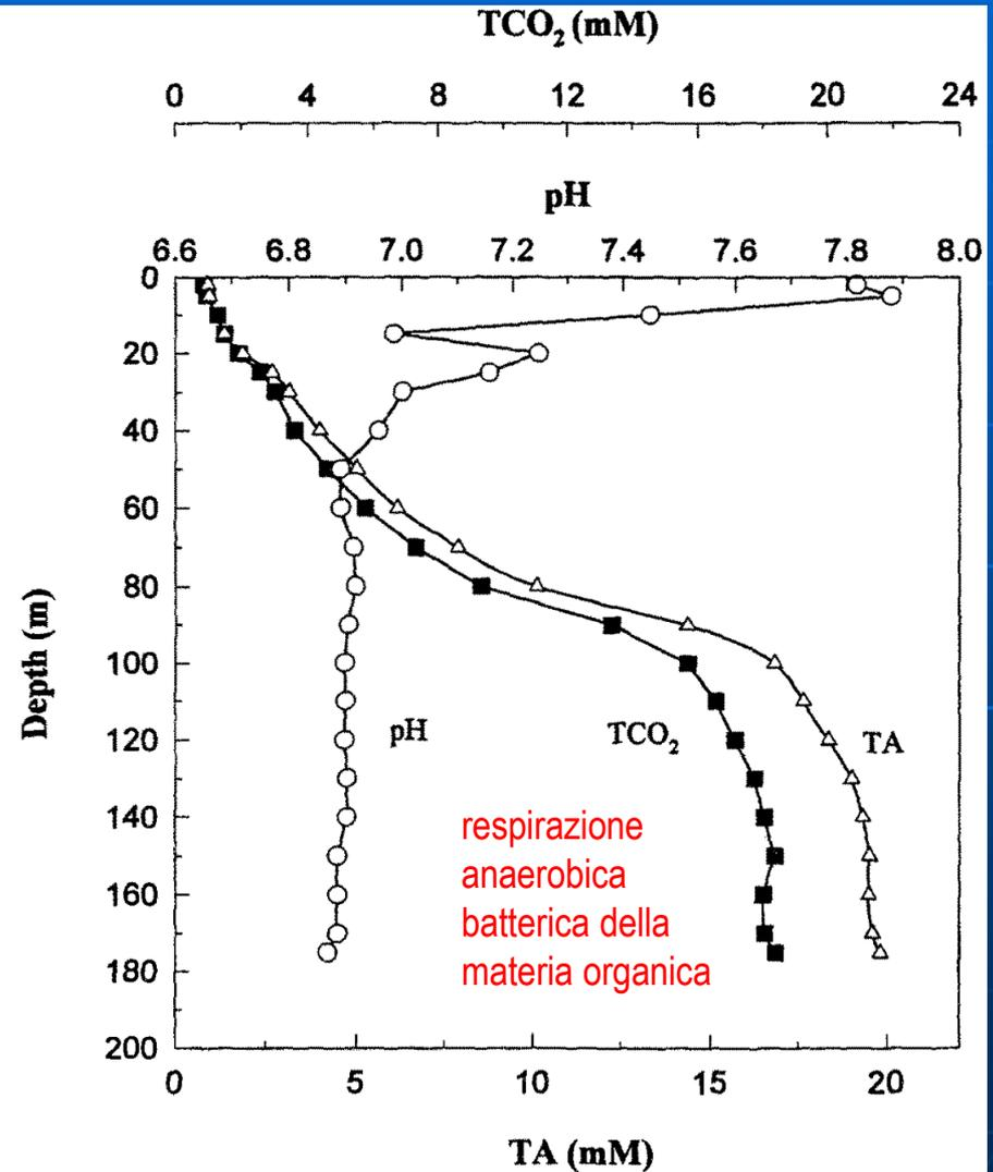
Fig. 4. Profiles of pH,  $\text{TCO}_2$  and TA in the Framvaren.
