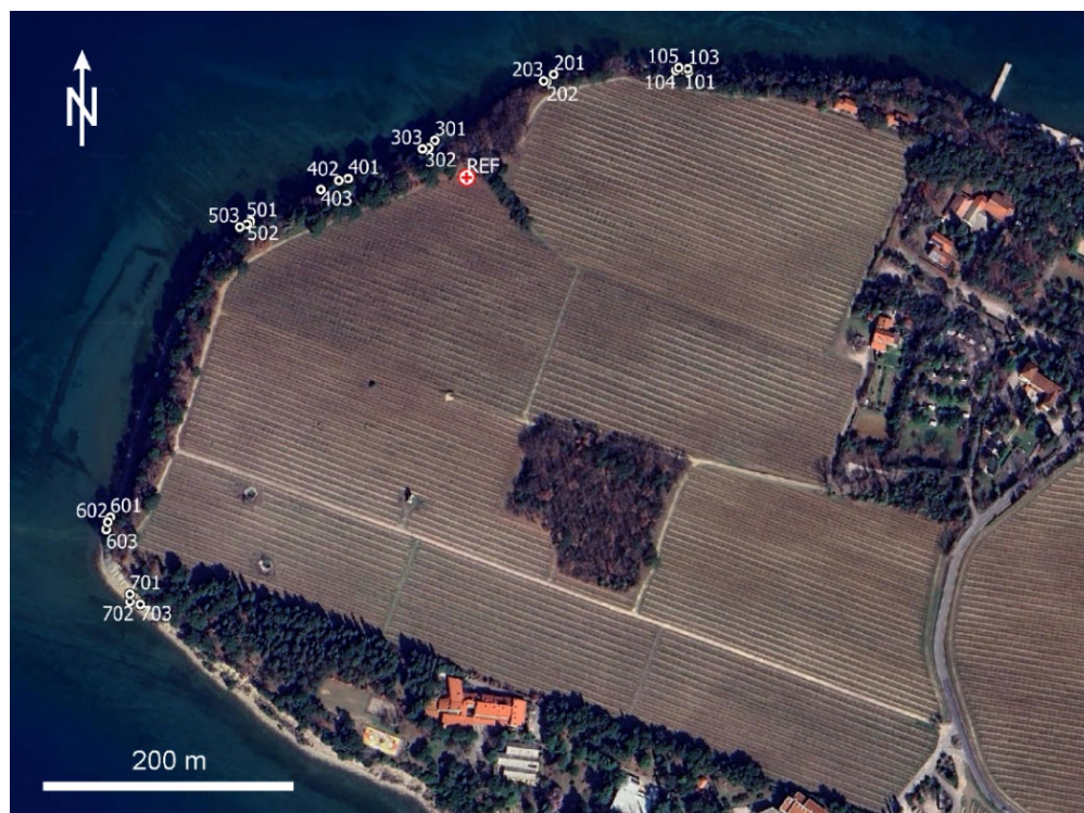
Figure 5. Spatial distribution of GCPs recorded with GNSS at some specific outcrops along the surveyed rocky coastline.
