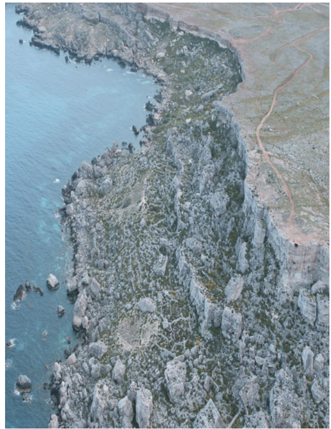
Fig. 2 The superimposition of the Upper Coralline Limestone Formation on the Blue Clay Formation is a predisposing cause of landslide occurrence along the north-west coast of Malta (Courtesy of Ten. Col. M. Marchetti)
