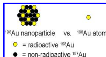
Figure 3. Schematic of gold nanoparticles made with ^{198}\text{Au} showing that more radioactive ^{198}\text{Au} is delivered per particle compared with a single ^{198}\text{Au} .
