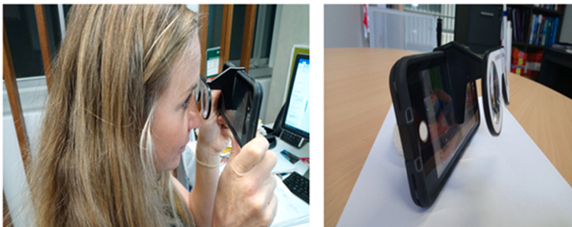
Fig. 2. Stereoscopic lenses and mobile phone set up for viewing the 3DMVR visualisation.
