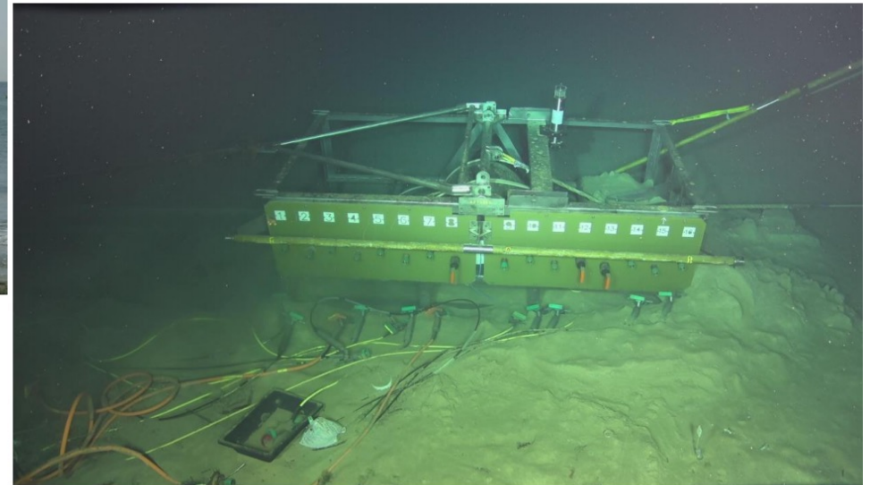
2002 Junction Box deployment: no failure in 20 years
