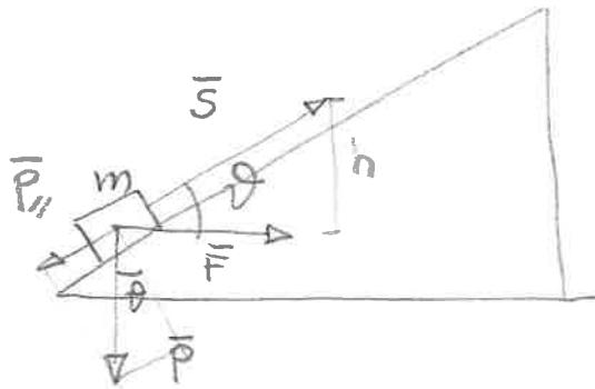
$$\begin{aligned} \theta &= 30^\circ \\ F &= 20 \text{ N} \\ m &= 3,0 \text{ kg} \\ s &= 50 \text{ cm} = 0,50 \text{ m} \end{aligned}$$
