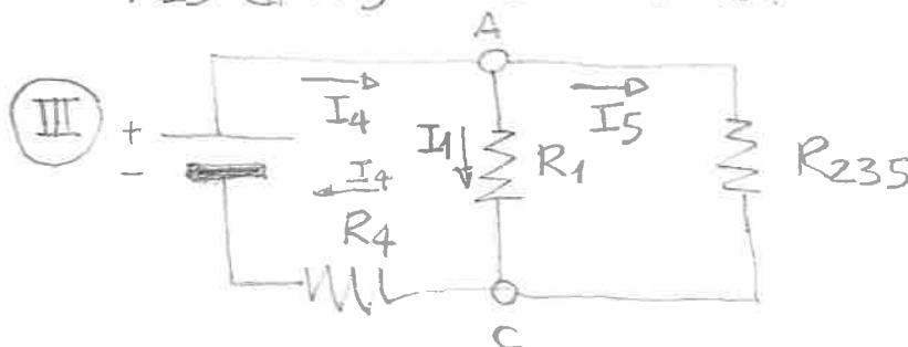
$$R_{235} = R_{23} + R_5 = \frac{R}{2} + \frac{5}{2} R = \frac{6}{2} R = 3R = 30 \Omega$$
