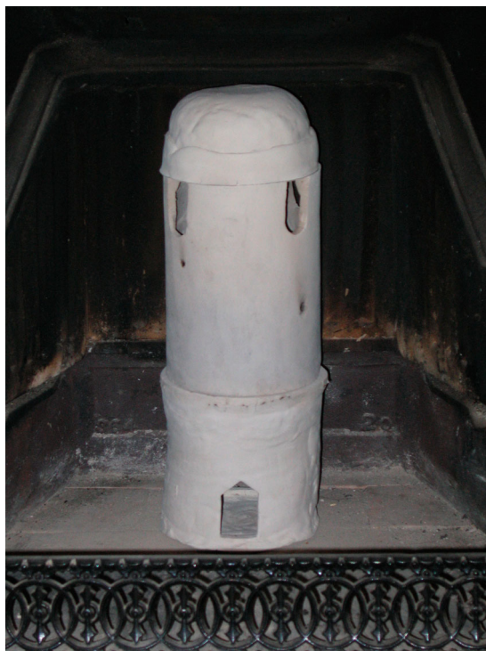
FIGURE 3 The special furnace for calcining the Bologna Stone, as reconstructed according to the directions and dimensions given by Wilhelm Homberg in 1687.
