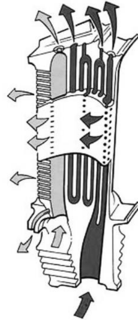
QUINTUPLE PASS, MULTI-FEED INTERNAL COOLING WITH EXTENSIVE FILM COOLING
