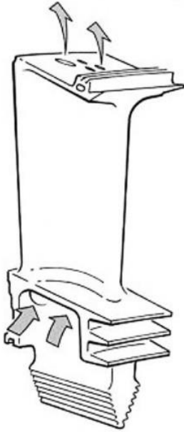
SINGLE PASS, INTERNAL COOLING (1960's)
