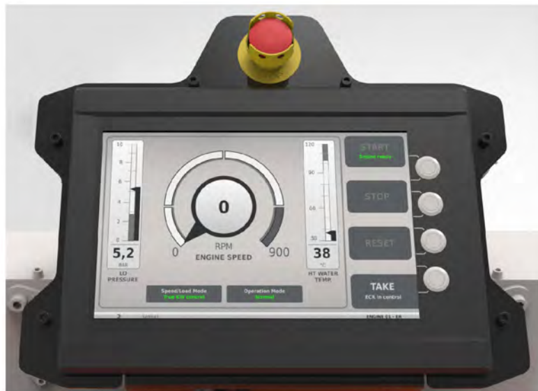
Fig 14-2 Local operator panel
