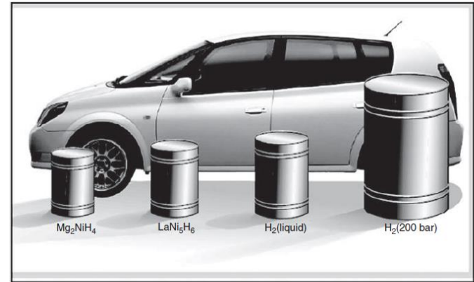
Figure 7.9 Alternatives for storage of 4 kg hydrogen with volume relative to the size of a car [32].
