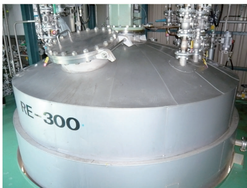
Figure 3. Menthol production at the Takasago Iwata Factory, Shizuoka. Top: The distillation towers for purification of geranyldiethylamine visited by R. Noyori (lower left-hand corner) in 1984. Bottom: The current (2012) reactor for the asymmetric 1,3-hydrogen shift reaction. Courtesy of the Takasago International Corporation.
