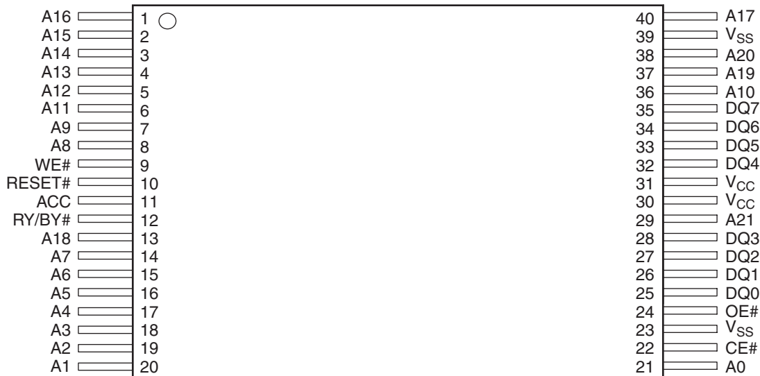
Figure 3.2 48-pin Standard TSOP
