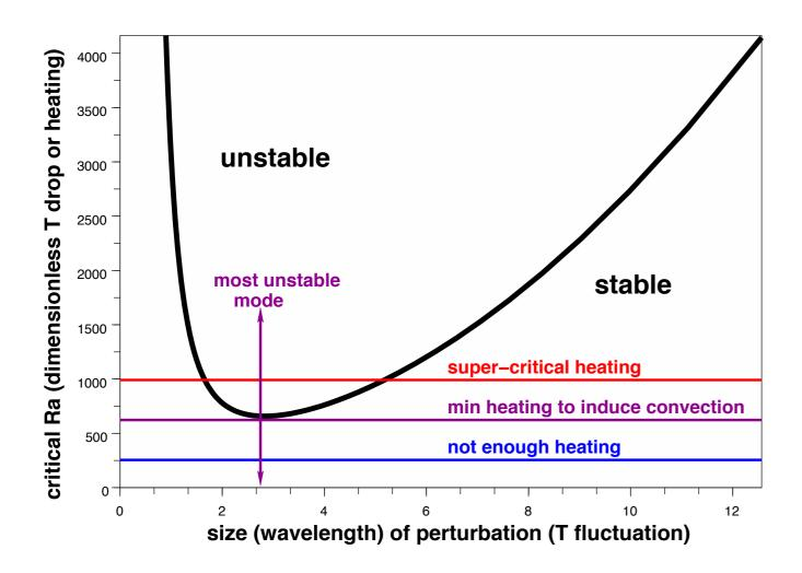
Values of Ra above the Ra<sub>c</sub> curve are associated with the conductive layer being convectively unstable (perturbations grow), while below the curve the layer is stable (perturbations decay). The minimum in the Ra<sub>c</sub> curve occurs at the wavelength of the first perturbation to go unstable as heating and Ra is increased, often called the most unstable mode.
