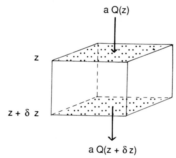
The net change in heat in the element is (heat entering across z) minus (heat leaving across  $z+\delta z$ ):
