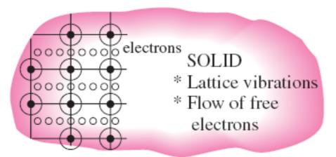
The mechanisms of heat conduction in different phases of a substance.
