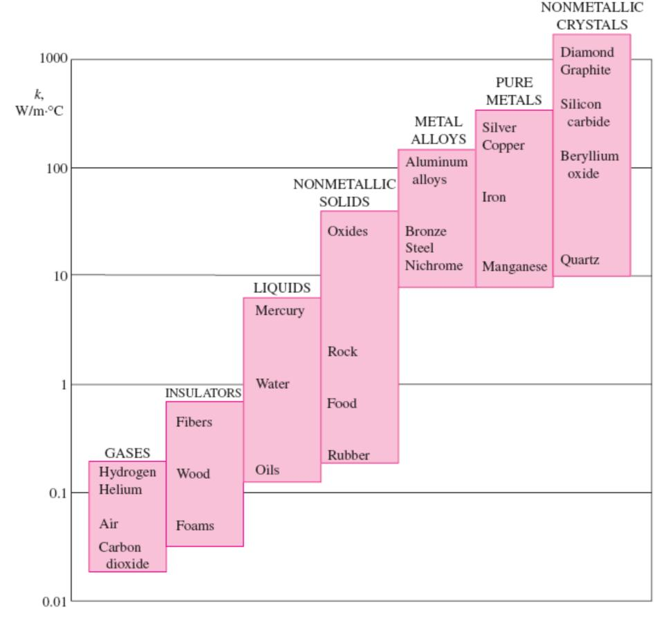
The range of thermal conductivity of various materials at room temperature.
