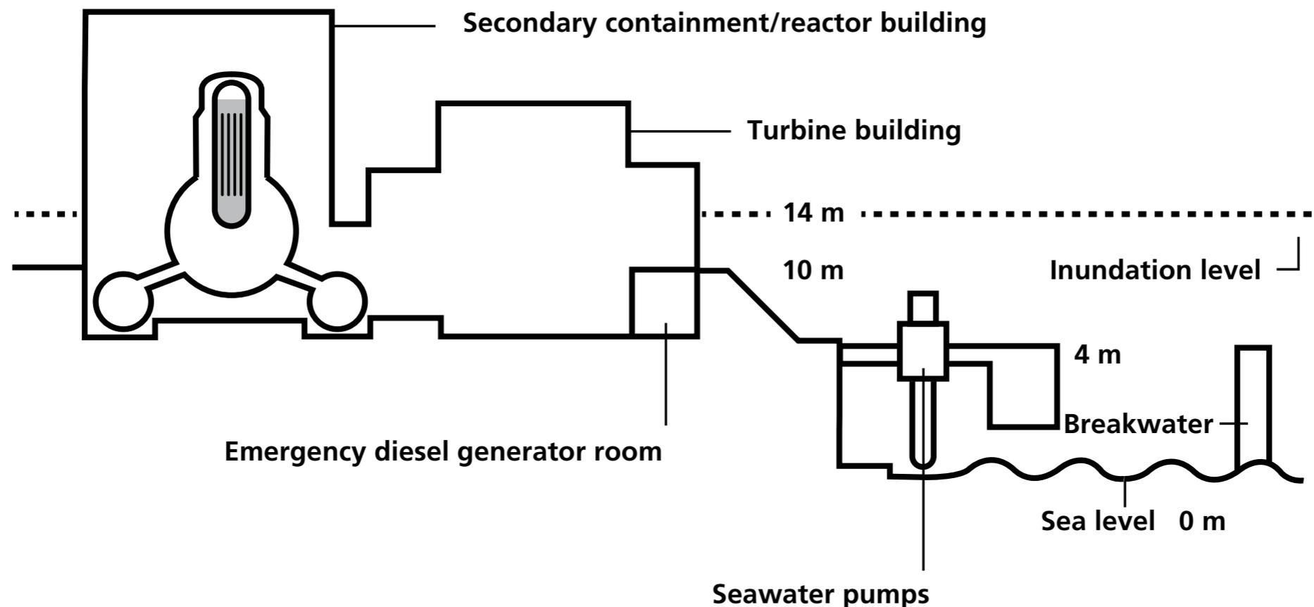
Simplified cross-section through one of the reactors at Fukushima Daiichi showing the approximate location of critical components damaged by the tsunami. Not drawn to scale.
