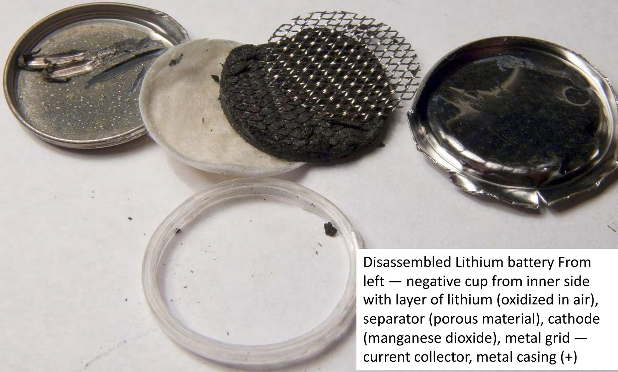
Disassembled Lithium battery From left — negative cup from inner side with layer of lithium (oxidized in air), separator (porous material), cathode (manganese dioxide), metal grid — current collector, metal casing (+)
