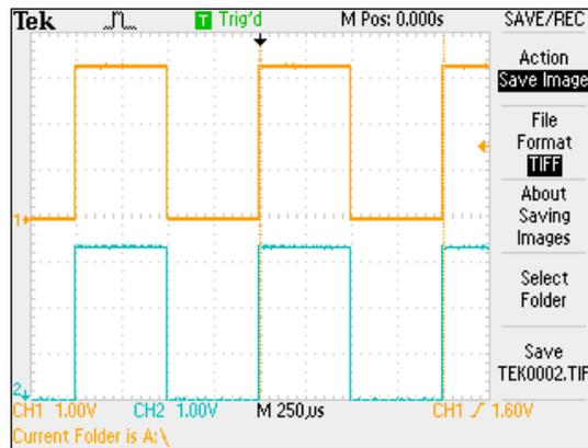
9. After a runtime of two seconds, the signals should disappear and both lines should be permanently zero. That is the result of the over current signal (GPIO18), which was generated after that time.
