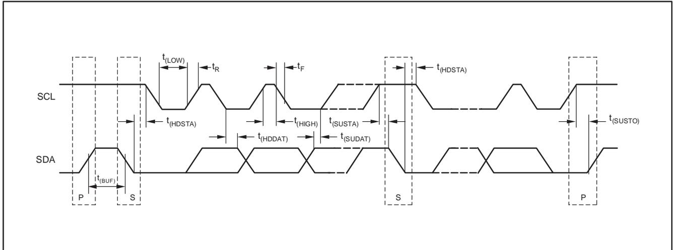
Figure 5. I<sup>2</sup>C Timing Diagram
