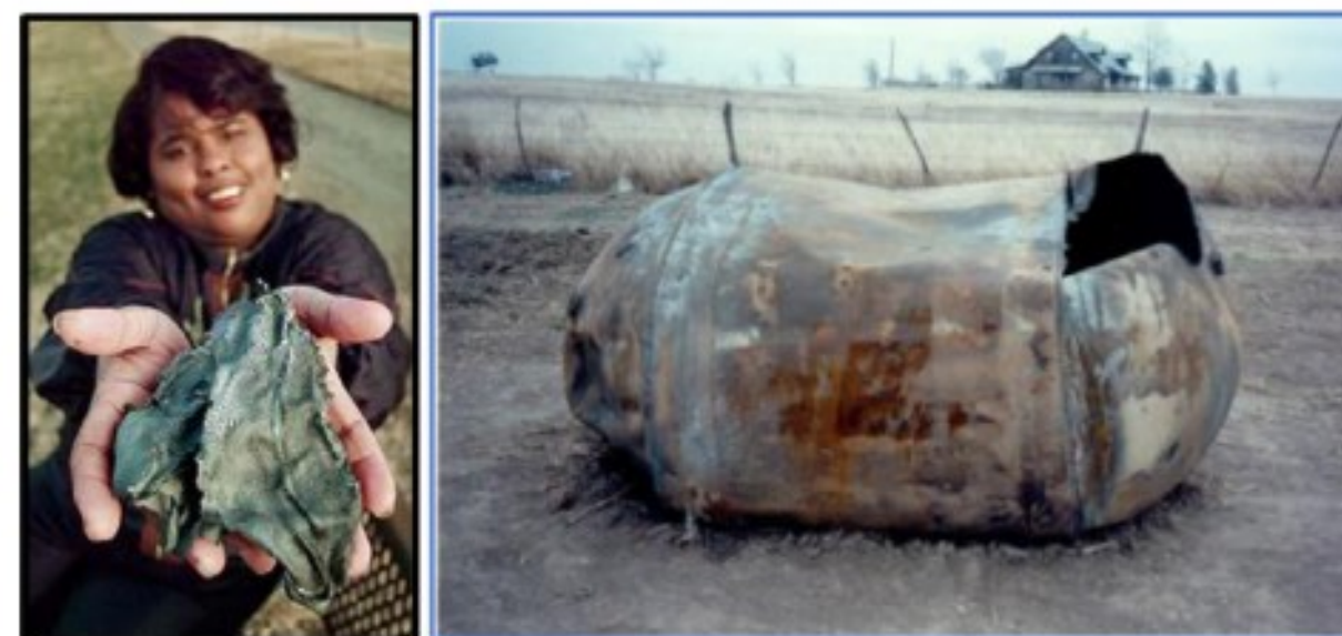
Fig. 5. Delta II State 2 debris: Left: Lottie Williams holding reentered debris fragment (photo courtesy Brandi Stafford, Tulsa World); Right, Propellant tank in Texas field (photo courtesy NASA).
