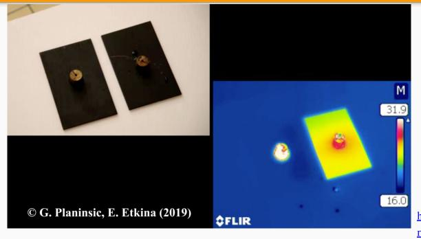
In the experiment, two identical metal objects (made of brass) are taken from the same hot water bath and placed on two identically-shaped (same height, length, and width) plates. The plates are made of wood and aluminum (colored with the same black paint to reduce the reflective properties of aluminum) and have been sitting on the table for a long time.
