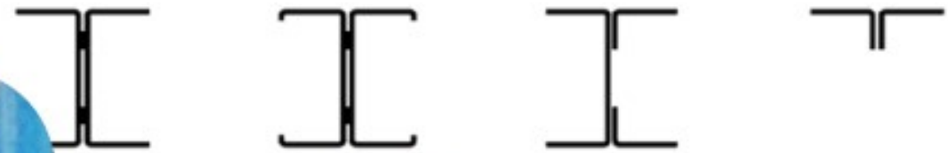
b) Open built-up sections
