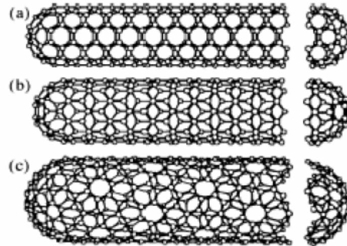
Some SWNTs with different chiralities. The difference in structure is easily shown at the open end of the tubes. a) armchair structure
