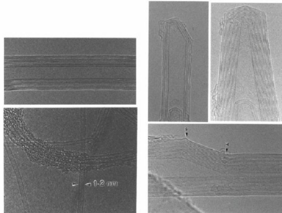
*Figure 1-4: Different structures of MWNTs. Top-left: cross-section of a MWNT the different walls are obvious, they are separated by 0.34nm. Rotation around the symmetry axis gives us the MWNT. Top-right: Symmetrical or non-symmetrical cone shaped end caps of MWNTs. Bottom-left: A SWNT with a diameter of 1,2nm and a bundle of SWNTs covered with amorphous carbon. Bottom-right: A MWNT with defects. In point P a pentagon defect and in point H a heptagon defect.<sup>6</sup>*
