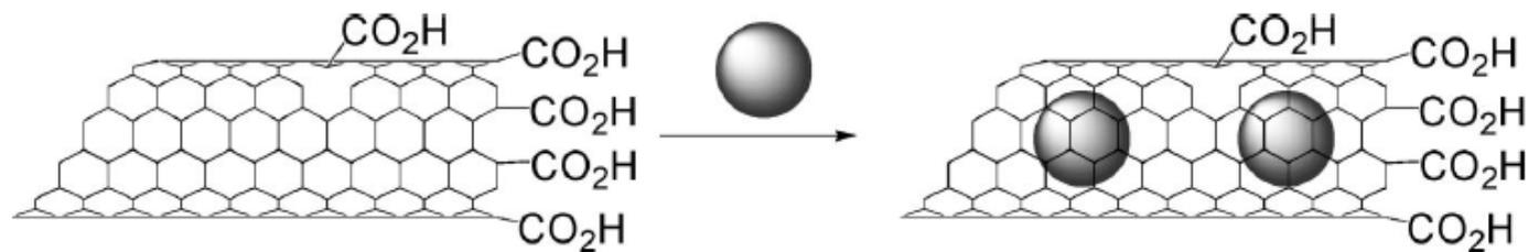
fullerenes, porphyrins, and metals, have indeed been included in the internal space of CNT, mostly due to hydrophobic interactions
