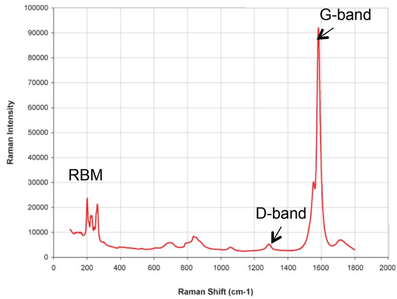
Raman spectrum of HiPCO SWCNTs using a laser wavelength of  $\lambda_{exc} = 633$  nm.
