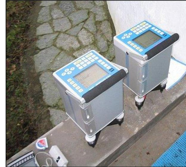
Gravimeters for general surveying use are capable of registering changes in gravity with an accuracy of 0.1 gu. A new generation of more efficient zero-length springs has been developed. Microprocessor-controlled instruments are now available which are, within limits, selflevelling, and which allow observations to be made rapidly. Also available for more specialized surveys are gravimeters capable of detecting gravity changes as small as 1 microgal ( $10^{-8}\text{ms}^{-2}$ ) !!!.
