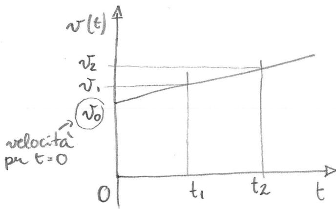
$$a_m = \frac{\Delta v}{\Delta t} = \frac{v_2 - v_1}{t_2 - t_1}$$
