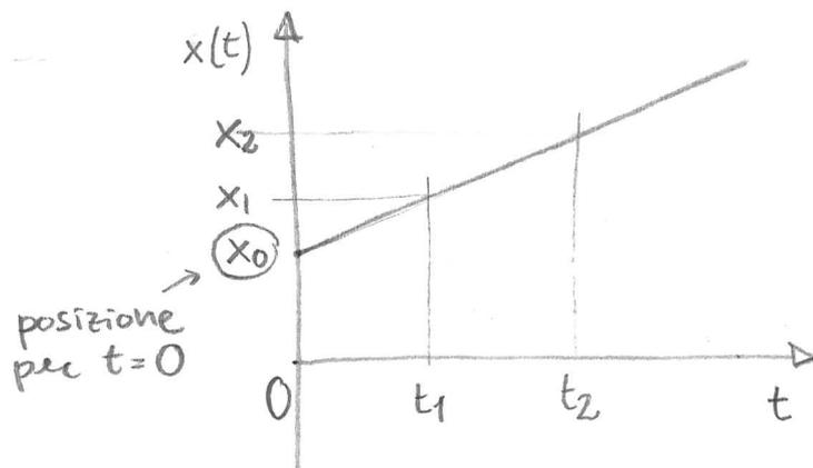
$$v_m = \frac{\Delta x}{\Delta t} = \frac{x_2 - x_1}{t_2 - t_1}$$
