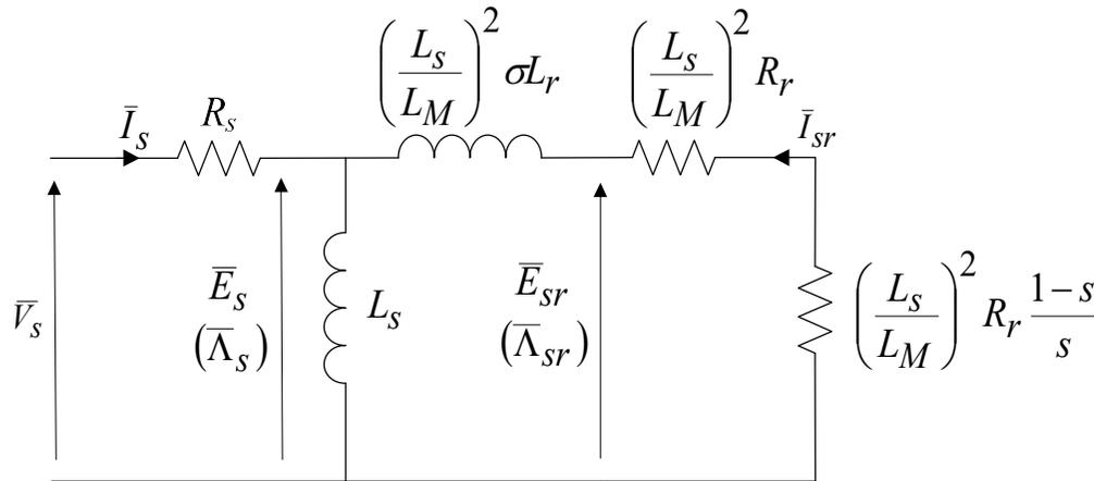
$$\bar{I}_s = \frac{\bar{\Lambda}_s}{L_s} + \frac{j\omega_s \bar{\Lambda}_s}{\left(\frac{L_s}{L_M}\right)^2 \left(\frac{R_r}{s} + j\omega_s \sigma L_r\right)}$$
