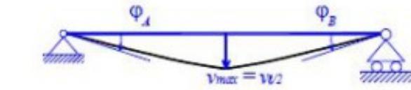
$$v_{\max} = v_{l/2} = \frac{F l^3}{48EI}$$
