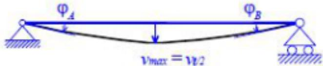
$v_{l/2} = \frac{5}{384} \frac{ql^4}{EI} = 0.0130 \frac{ql^4}{EI}$ $\varphi_B = -\varphi_A = \frac{ql^3}{24EI}$ |
