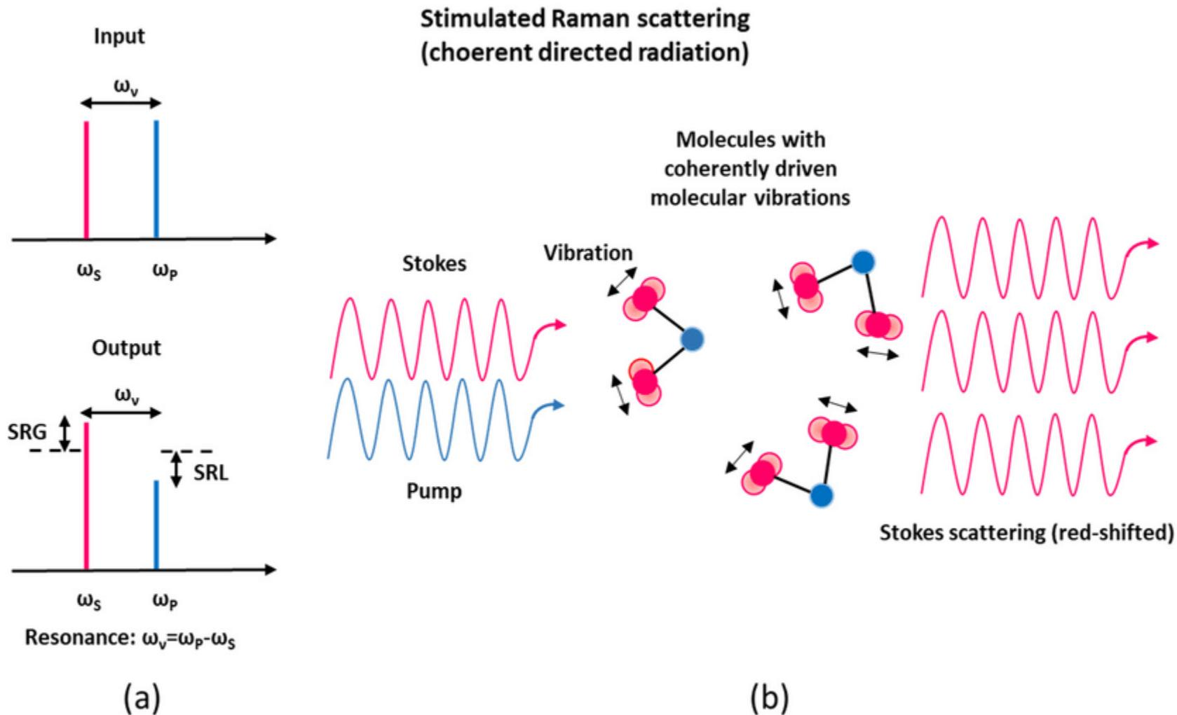
Stimulated Raman-Scattering (StRS) principle. (a) Pump-probe modalities associated with the SRS process are pointed out: SRG, stimulated Raman gain; SRL, stimulated Raman loss. (b) Stimulated Raman scattering occurs through inelastic scattering of probe photons off from vibrationally excited molecules that interfere coherently.
