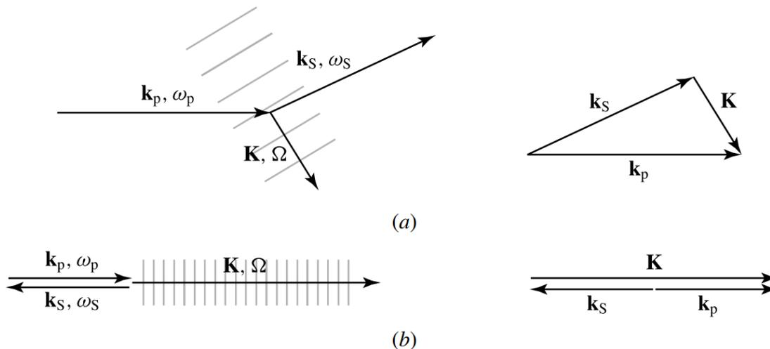
phase matching among the pump wave, the Stokes wave, and the material excitation
