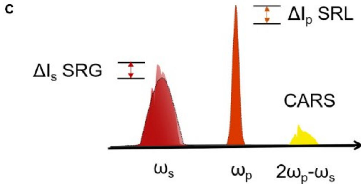
Schematic representation of the excitation and emission frequencies involved in StRS and CARS: in evidence the StRS signal in terms of gain (SRG) on the Stokes pulse or the loss (SRL) on the pump pulse.
