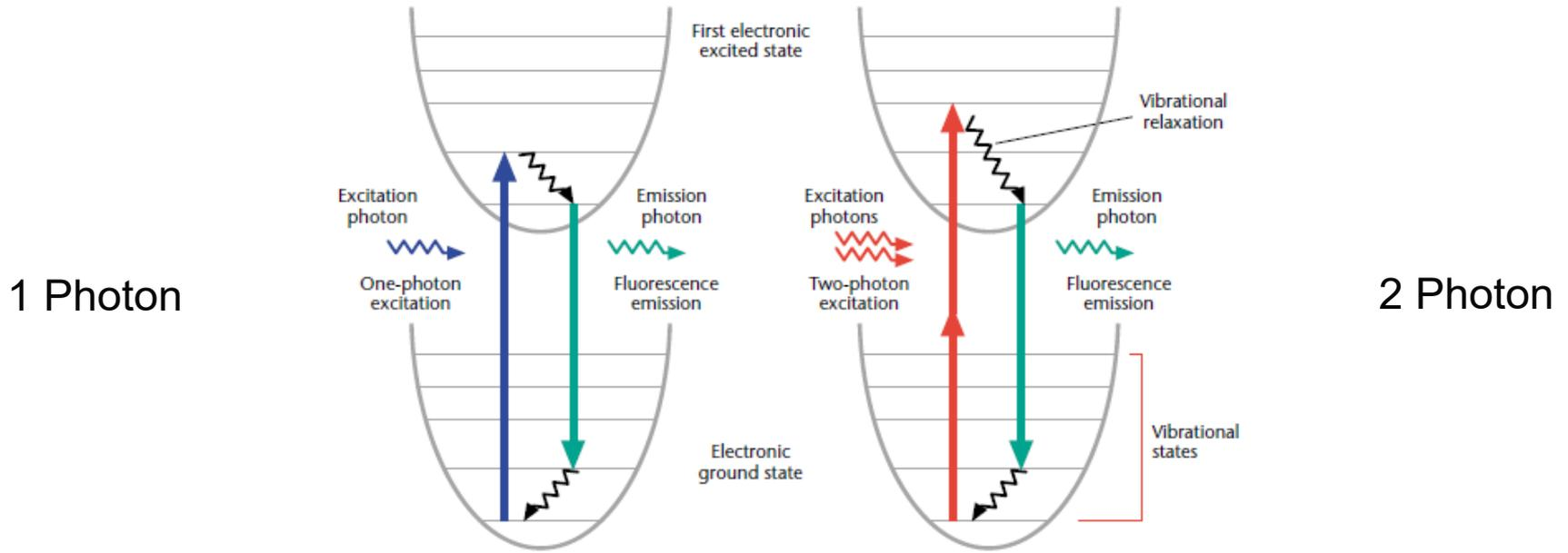
Two-photon excitation is a fluorescence process in which a fluorophore is excited by the simultaneous absorption of two photons.
