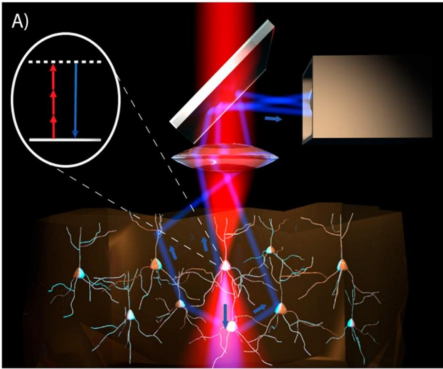
Schematic of THG microscopy on brain tissue in an epi-detection geometry.
