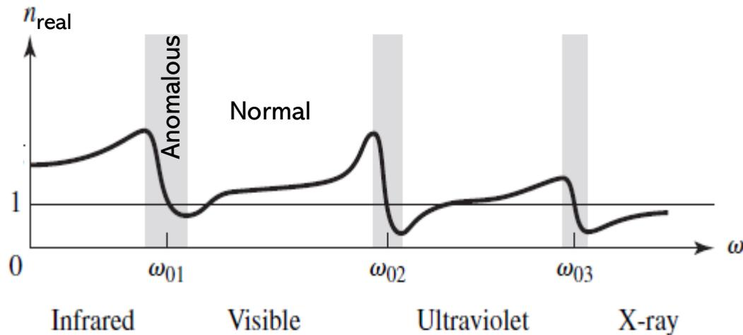
Dispersion - absorption around a resonance frequency
