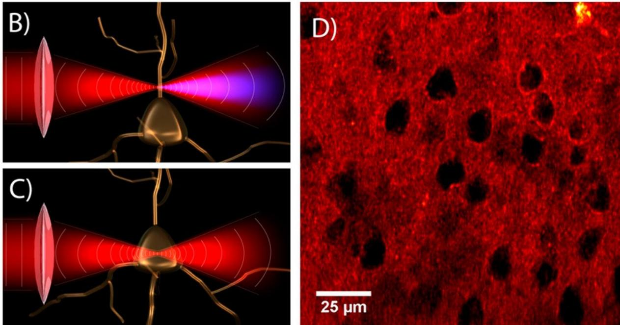
(B) Focused laser beam at a dendrite. By setting the laser focal volume several times larger than the dendrite diameter, partial phase matching is achieved, and a significant THG signal is produced.
