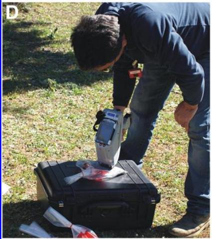
XRF set up for field analysis
