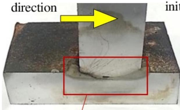
Fatigue fractures initiating at edge of weld HAZ
