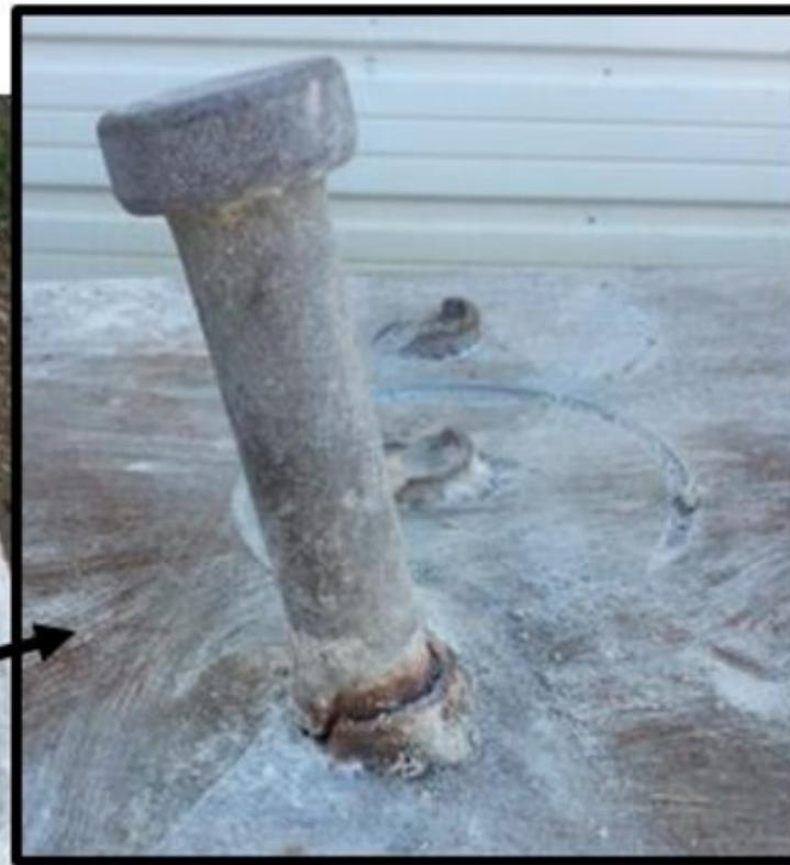
Failed Shear Studs remained embedded in Concrete Deck
