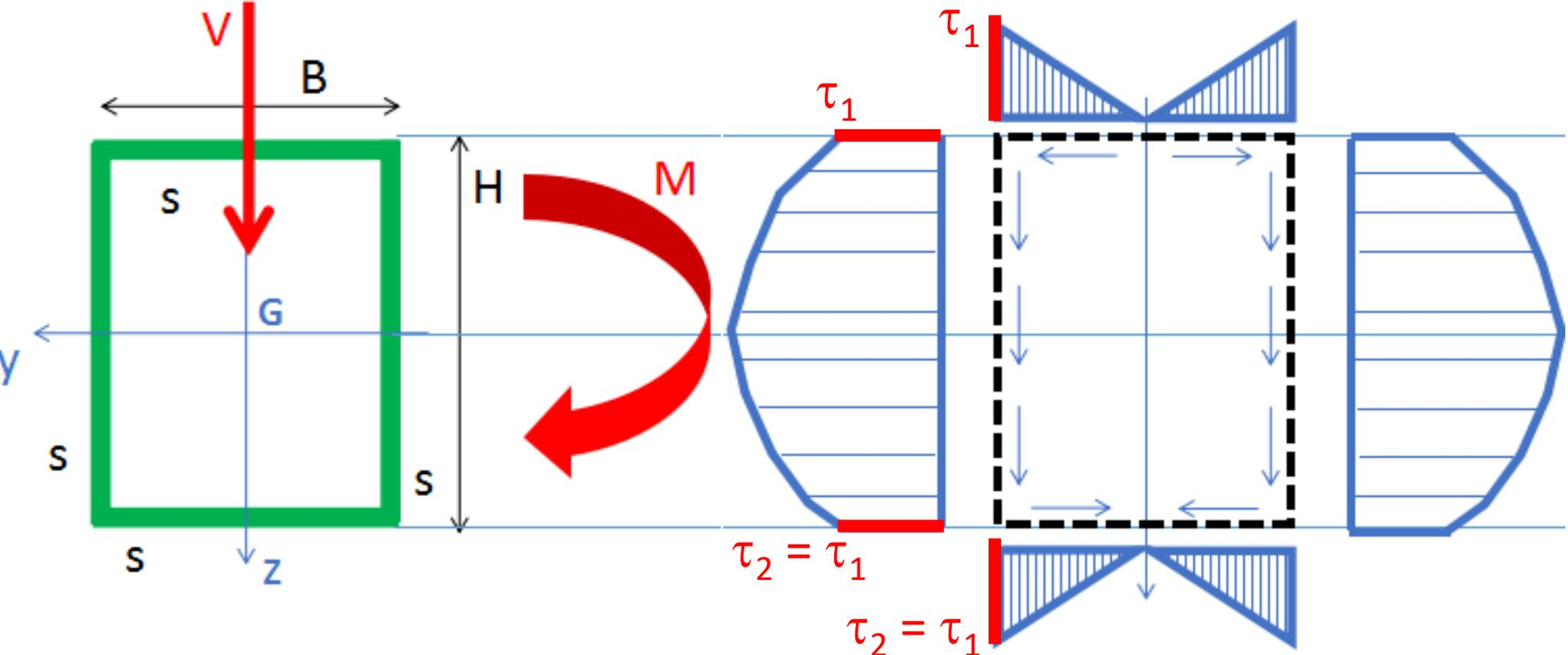
$$\begin{aligned} \tau_1 &= (V / J_y) \times (S_y / b) = \\ &= ((20 \times 10^3) / (3.29 \times 10^6)) \times (13500 / 10) = \\ &= 8.20 \text{ MPa} \end{aligned}$$
