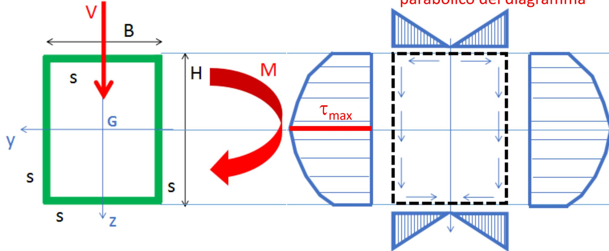
$$\begin{aligned}\tau_{\max} &= \tau_1 + \Delta\tau = \\ &= 8.20 + 4.86 = \\ &= 13.06 \text{ MPa}\end{aligned}$$
