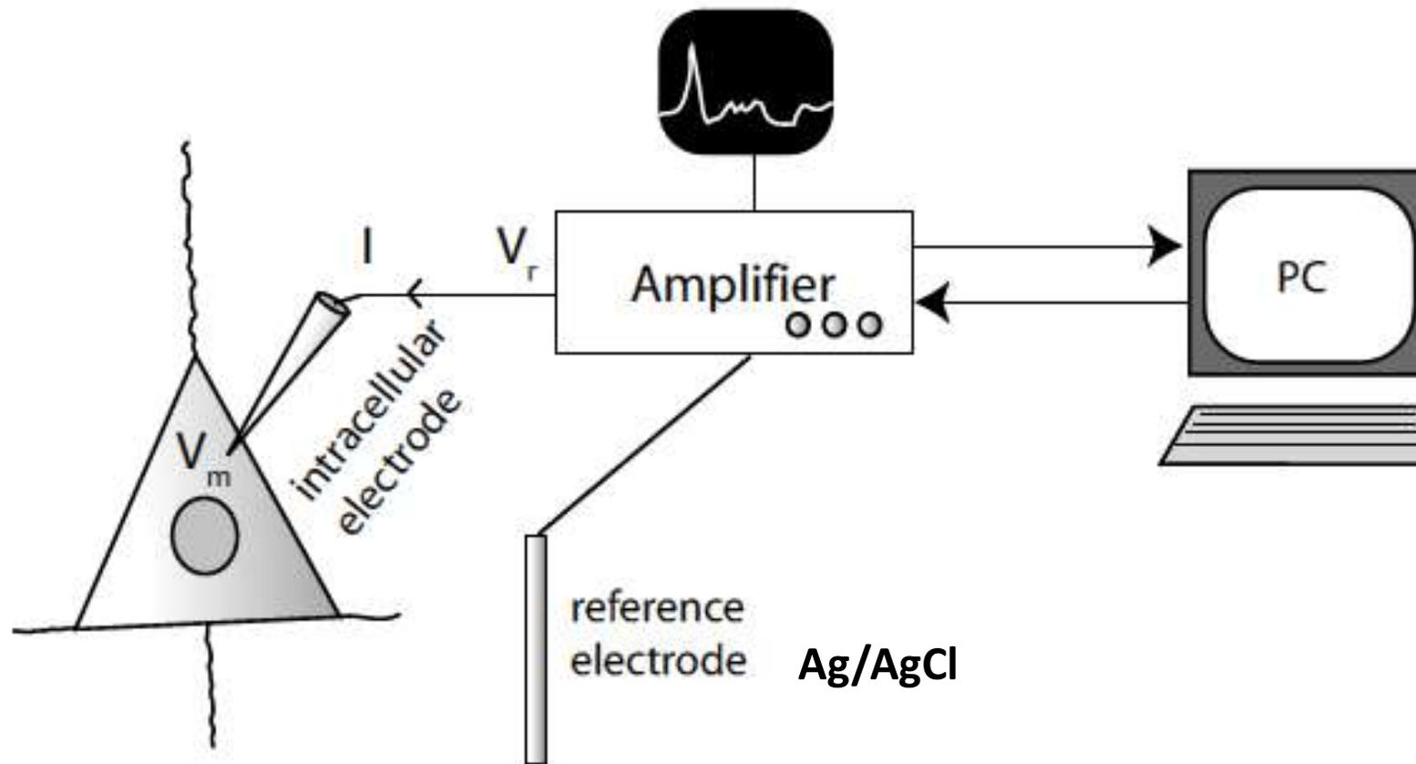
Basic intracellular experimental setup. An intracellular “sharp” microelectrode is impaled into the cell and connected to an amplifier, which records the intracellular membrane potential relative to that of a reference “bath” Ag/AgCl electrode.
