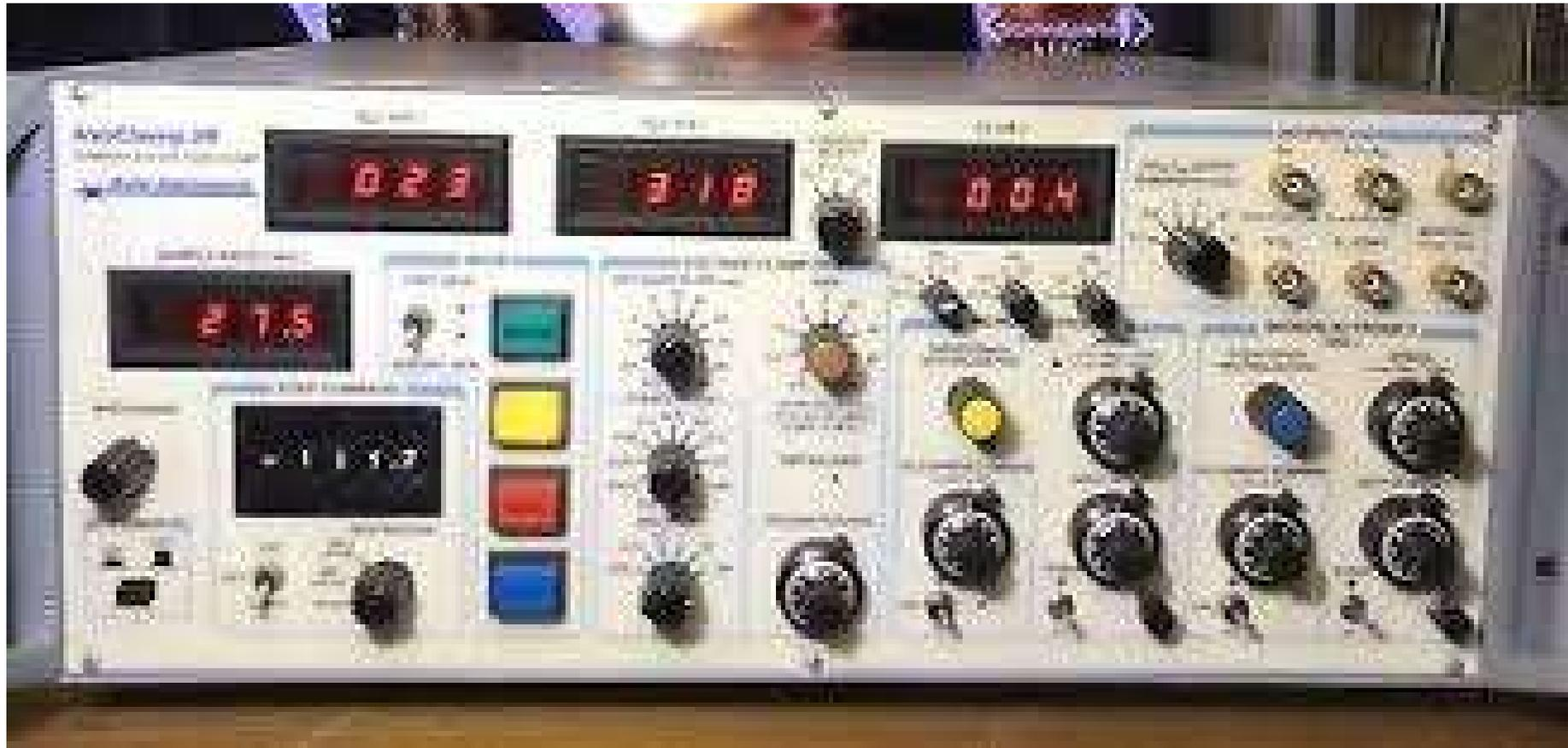
**Axon Instruments Axoclamp 2B discontinuous current clamp/voltage clamp recording preamplifier:**
