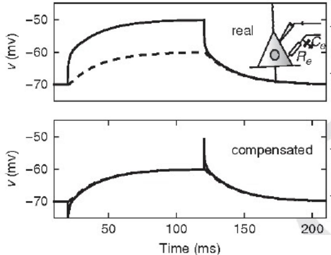
Upper trace shows intracellular electrotonic voltage response of a cell + microelectrode resistance artefact recorded following injection of a rectangular depolarizing current pulse. Lower trace shows the same response after bridge balance compensation for the microelectrode resistance  $R_e$ . This is **current clamp** recording.
