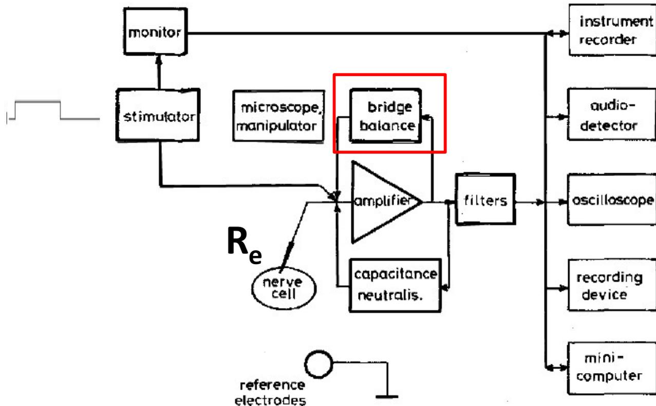
An intracellular “bridge balance” amplifier allows for intracellular current pulses to be injected into the cell to assess membrane excitability and input resistance. Passing current through the microelectrode resistance  $R_e$  will however generate a voltage artefact that adds on to the real neuronal electrotonic response, therefore needs to be cancelled using a “bridge balance” circuit.
