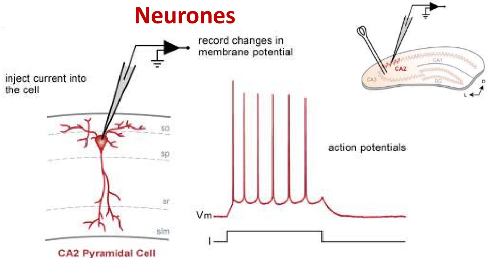
Intracellular recordings using “sharp” microelectrodes can also be made from brain slice neurones *in vitro*. The electrode is impaled into the cell and connected to a “bridge”-type amplifier, which records membrane potential and passes intracellular current pulses into the cell to record intrinsic excitability.
