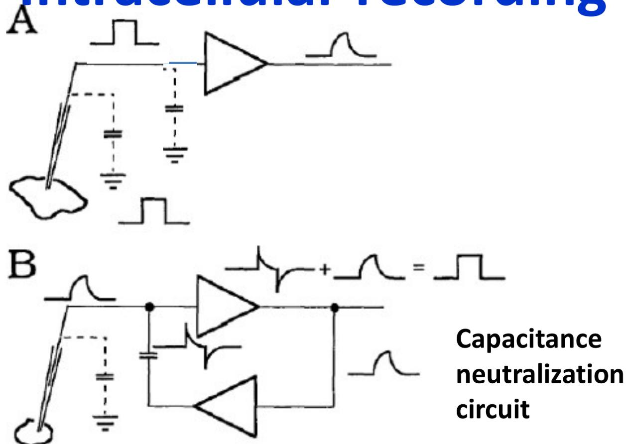
(A) The input capacitance of the amplifier and the microelectrode capacitance combine with the electrode resistance to form a low-pass filter that attenuates the high-frequency components of the measured signal. (B) A capacitance neutralization feedback amplifier can restore the lost high-frequency components.
