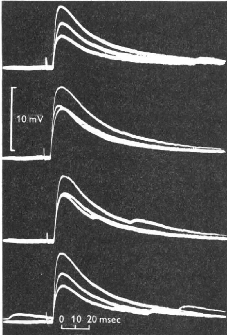
Fluctuation of evoked e.p.p. response at a single frog NMJ, treated with 10 mM-Mg<sup>2+</sup> + 10<sup>-6</sup>M prostigmine (anticholinesterase). In each record, three superimposed responses are seen. Note variation in amplitudes and scattered spontaneous miniature potentials. From Del Castillo & Katz (1954). Quantal components of the end-plate potential *J. Physiol.* 124(3):560-573.
