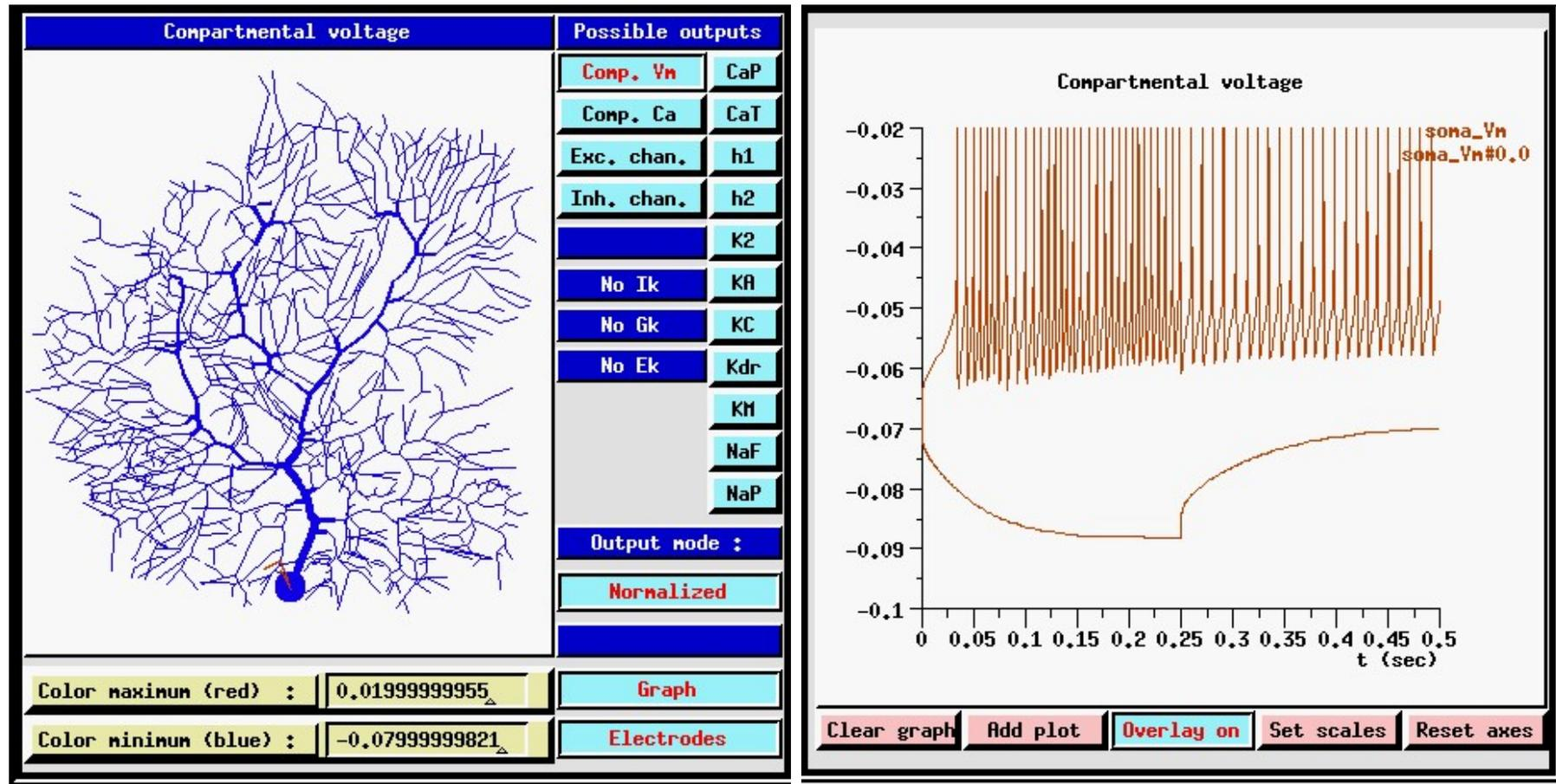
The Figure shows a cerebellar Purkinje cell model run on the **GENESIS** simulation program, with a current injection pulse applied to the soma. The plots show the superimposed results of  $\pm 1$  nA current pulses.
