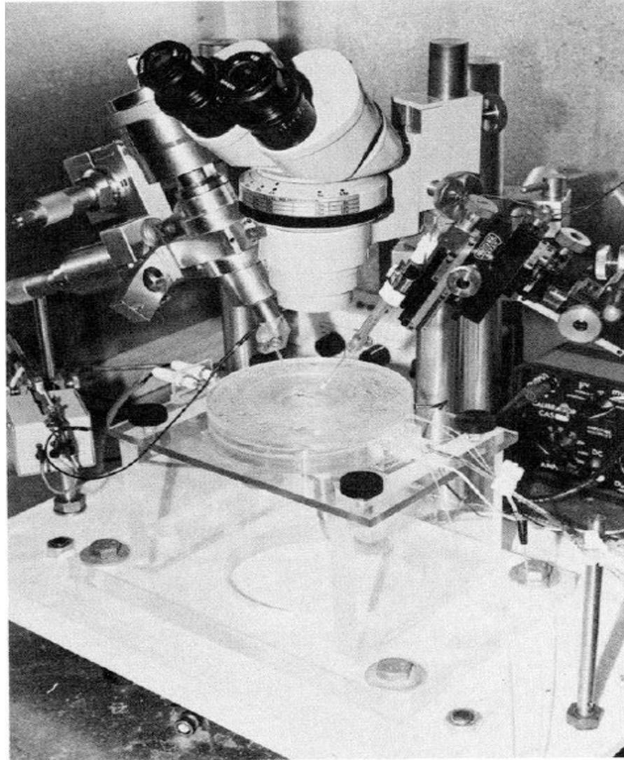
Photograph of a typical *in vitro* brain slice recording set-up.
