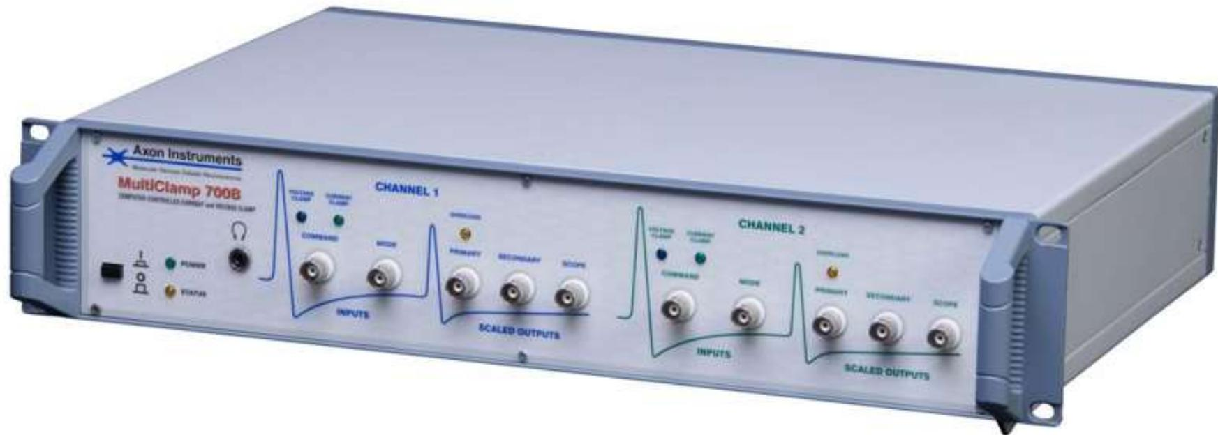
The Axon Instruments MultiClamp™ 700B Microelectrode Amplifier is a more modern versatile, computer-controlled microelectrode amplifier designed for patch voltage-clamp or high-speed current clamp (sharp-electrode) recording within the same headstage.
