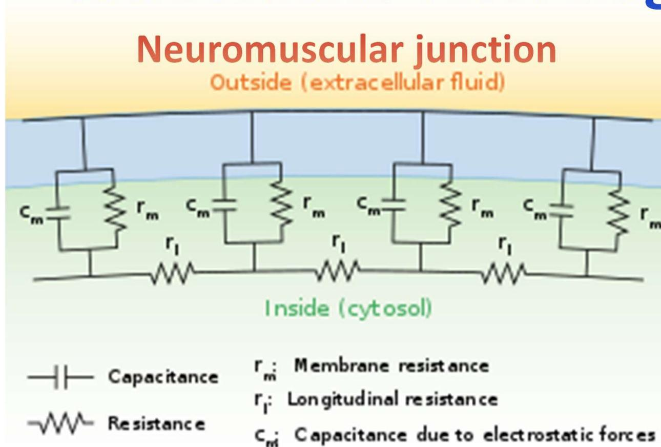
Cable theory's simplified electrical representation of a muscle fibre as an "infinite cable" .
