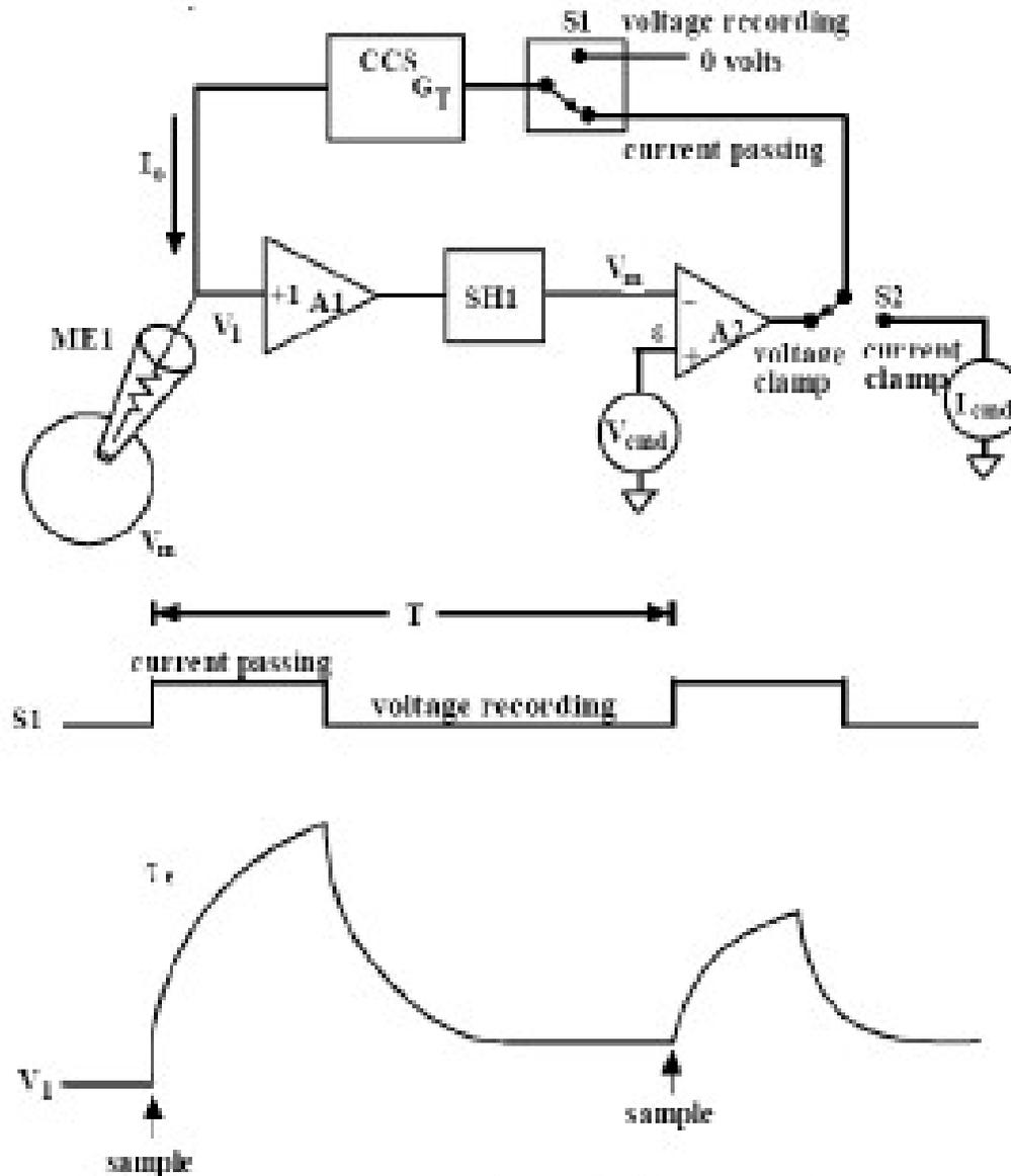
Circuit diagram showing principle of **discontinuous current clamp**, current injection/voltage recording preamplifier.
