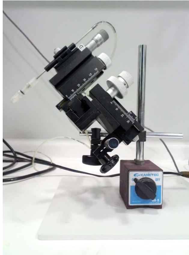
A more advanced micromanipulator positioning system is usually preferred for making stable intracellular neuronal recordings, sometimes using a motorised or electromechanical (piezoelectric) control stage making fine step movements through the tissue.
