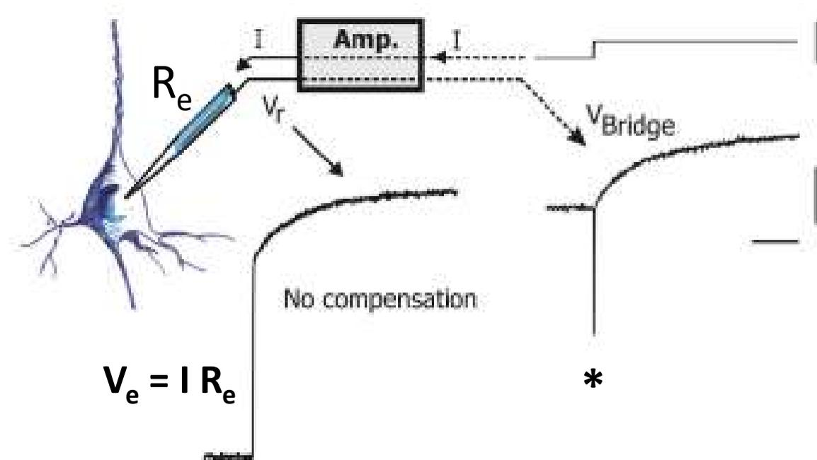
With standard bridge balance compensation, the accuracy of measurements can change if the electrode resistance  $R_e$  changes during the recording. Electrode capacitive transients (\*) are also present at the make and break of the injected current pulse.
