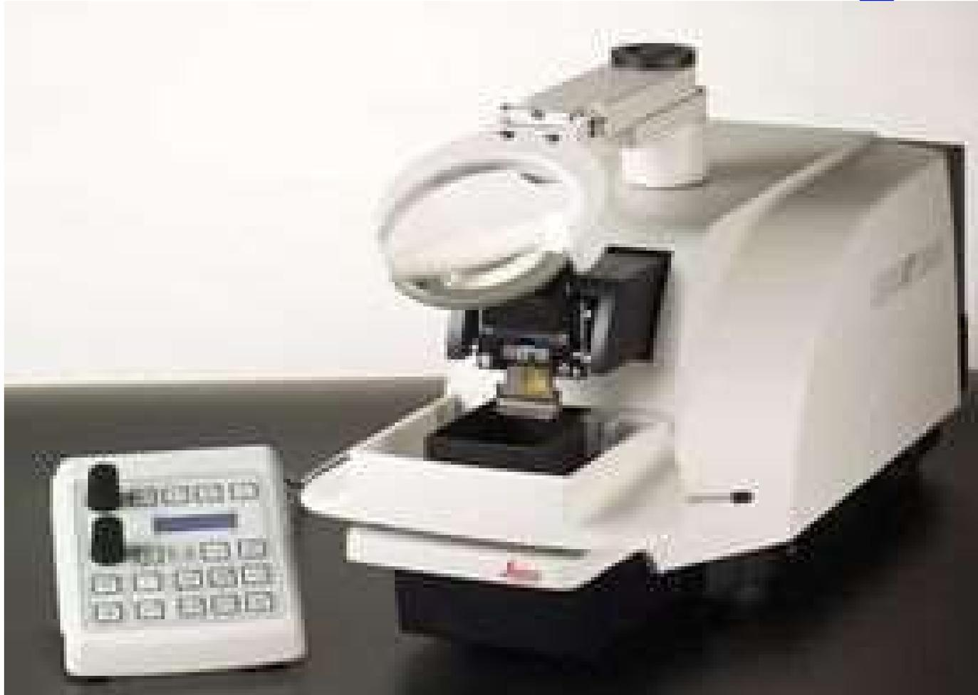
**Leica VT1200 S** : A vibrating blade “vibroslice” tissue cutter for preparing acute brain slices for recording.
