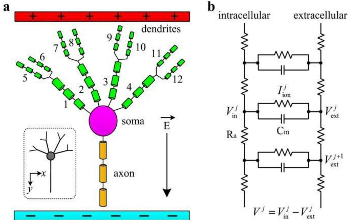
Artificial pyramidal neurone. (a) Schematic diagram of the multi-compartment artificial model simulated by the **NEURON** modelling program. (b) Circuit representation of the active compartments. From Yi et al., (2017) *Scientific Reports*, 7: 3210.
