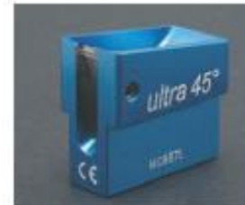
Ultra Used in room temperature. For thin sectioning.
