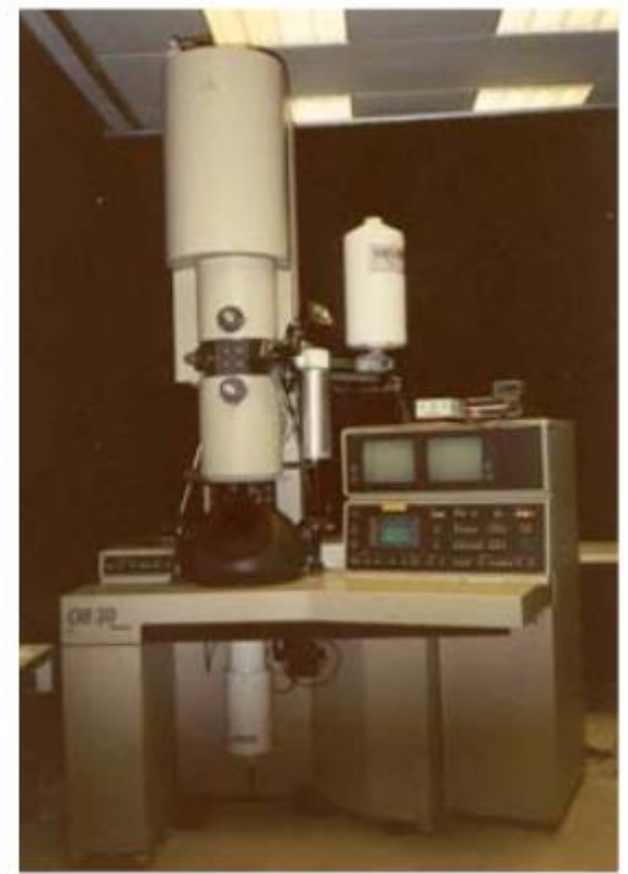
~1990 Philips CM30, V = 300 kV resolution ca. 0.2 nm
