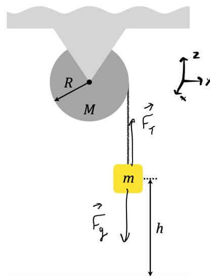
$$U_i + K_i = U_f + K_f \rightarrow mgh = \frac{1}{2} m v_f^2 + \frac{1}{2} I \omega_f^2$$
