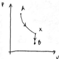
$$A \rightarrow X : \Delta S = n R \ln \left( \frac{V_X}{V_A} \right) \quad V_X = V_B$$
