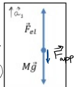
$$\underbrace{\sum \vec{F}_{real}}_{\vec{F}_{el} + M\vec{g}} + \underbrace{\sum \vec{F}_{app}}_{\vec{F}_{app} = -M\vec{a}_{inert} = -M\vec{a}_1} = M \vec{a}' = 0 \Rightarrow \vec{F}_{el} + M\vec{g} - M\vec{a}_1 = 0$$
