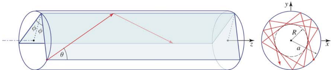
Figure 10.1-2 A skewed ray lies in a plane offset from the fiber axis by a distance R . The ray is identified by the angles \theta and \phi . It follows a helical trajectory confined within a cylindrical shell with inner and outer radii R and a , respectively. The projection of the ray on the transverse plane is a regular polygon that is not necessarily closed.
