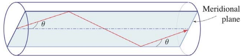
Figure 10.1-1 The trajectory of a meridional ray lies in a plane that passes through the fiber axis. The ray is guided if \theta < \bar{\theta}_c = \cos^{-1}(n_2/n_1) .
